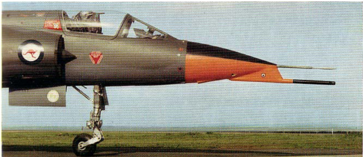
Figure 3: Gust Probe Mounted to Flight Trials Aircraft
