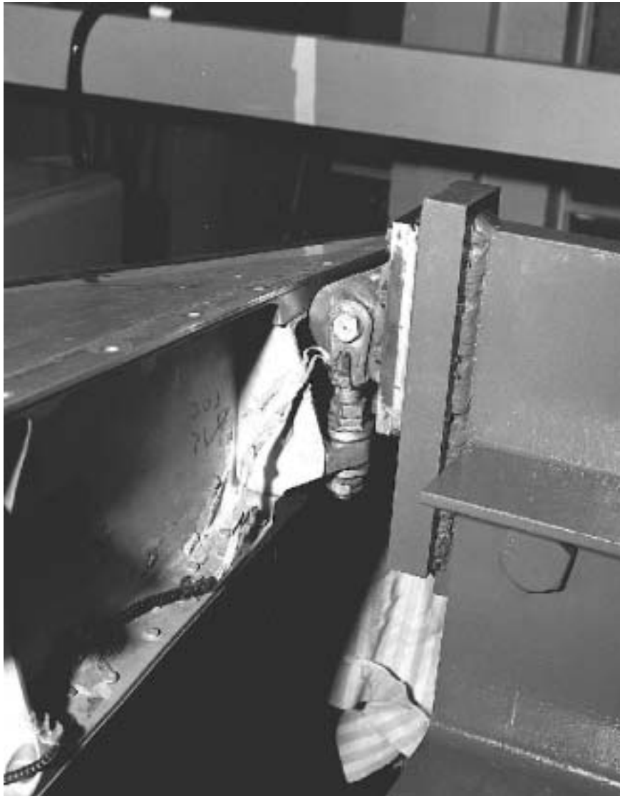
Figure 33: Leading Edge Attachment to Dummy Fuselage
