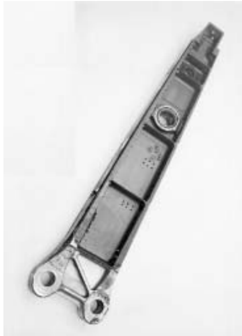
Figure 9: Aft Side of Starboard Main Spar Showing Diagonal Brace
