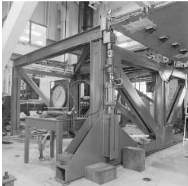
Figure 30: Wing Test Rig Dummy Fuselage Showing Two of Four Attachment Locations
