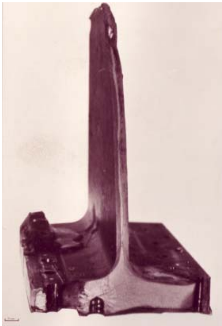
Figure 27: General View of the Final Failure in the Main Spar Lower Flange
