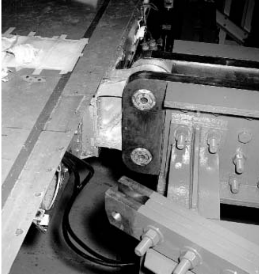
Figure 32: Main Spar and Undercarriage Side Link Attachment Points on Dummy Fuselage
