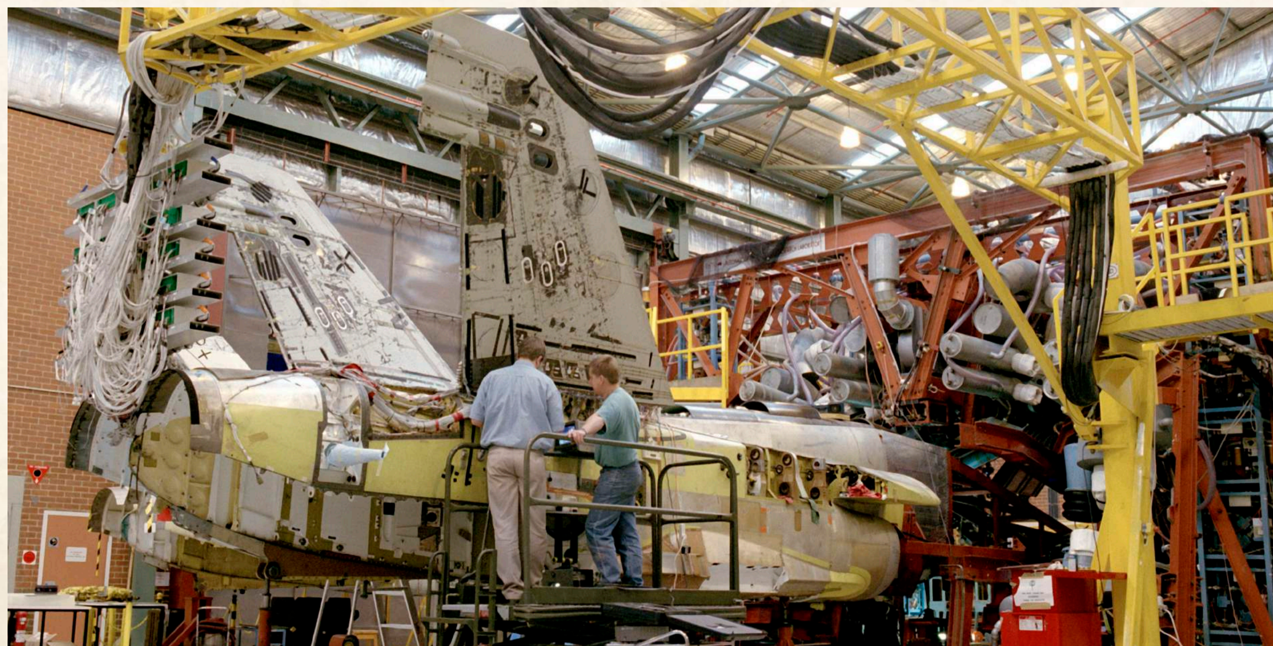
Full-scale structural fatigue test of the F/A-18 Hornet, known as IFOSTP, the International Follow-on Structural Test program
