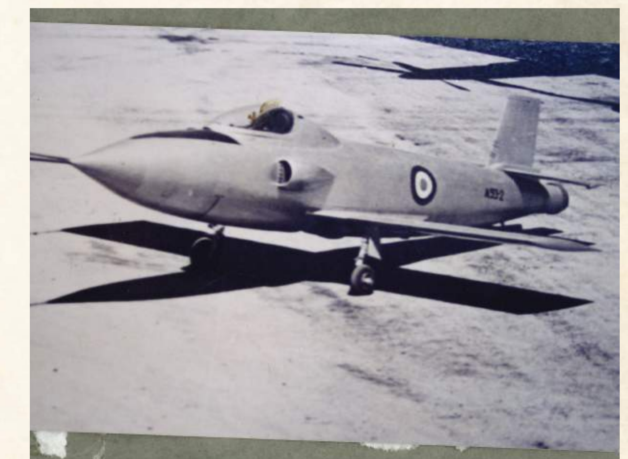
Jindivik - jet-propelled target plane
