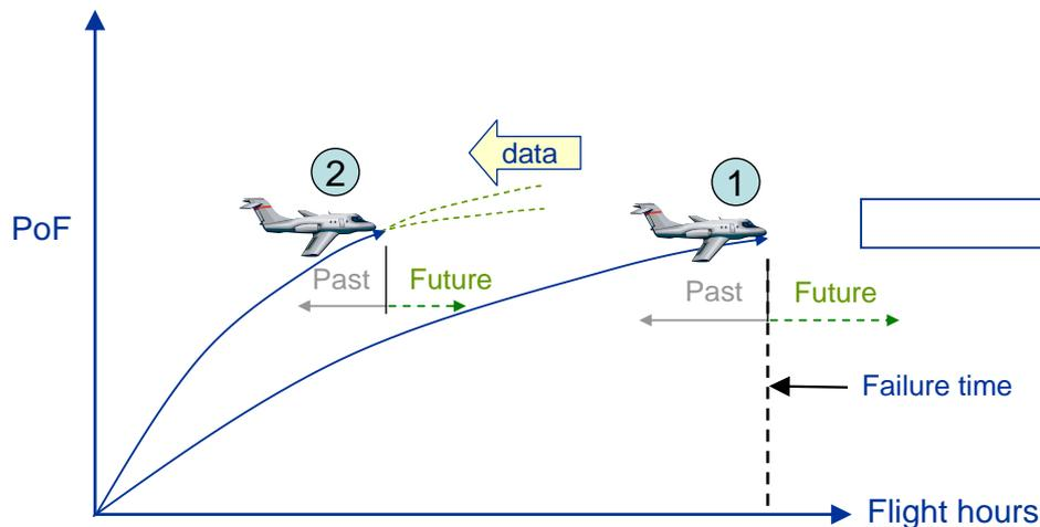
Case 2: Failure observed in one member of the fleet
