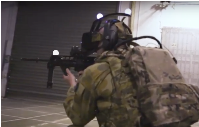
Fig. 1. Photo of a participant engaged in a FRVR tactical training. LCD markers attached to the HMD and to the simulated weapon allow tracking of the body and the weapon position. Backpack contains a computer that is wirelessly connected to a central server and generates VR for the HMD.
