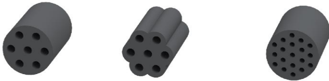
Figure 3. Conventional extruded propellant grain geometries, from left to right: 7-perforated cylinder; 7-perforated rosette; and 19-perforated cylinder.
