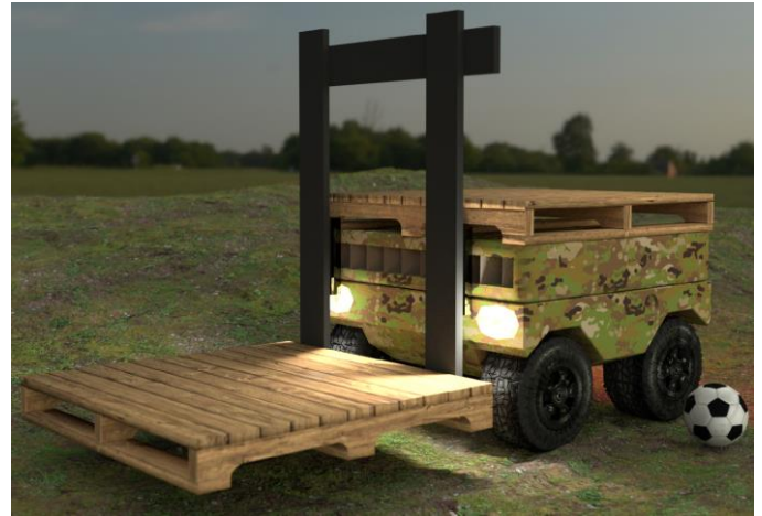
Fig. 2. A preliminary design for the off-road base carrying two pallets, with soccer ball for scale.
