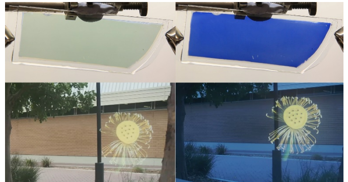
Fig. 5. The early prototype of AR headset contrast control device (photographed through Epson BT-200 AR glasses), demonstrating improvement of the augmented image contrast (a flower) in the outdoor application
