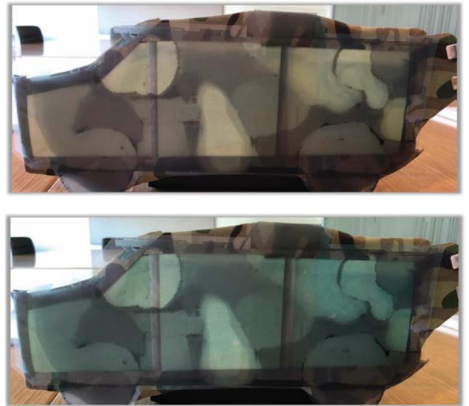
Fig. 4. The outline of the Bushmaster PMV with active camouflage panels and shade rendering mask, in two colour states.
