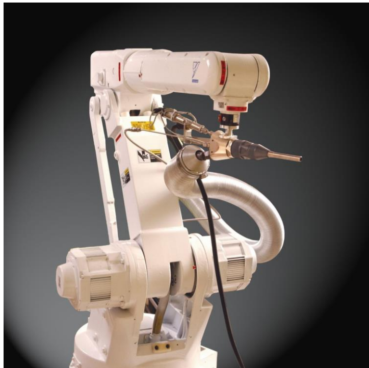
Figure 1. Spray nozzle on a robotic arm for complex additive deposition at Lab 22 (Copyright CSIRO, 2016).
