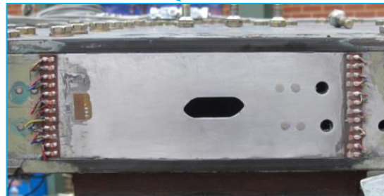
Outer wing front spar grounding hole
