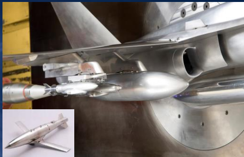
Wind Tunnel Model of F/A-18A/B and JDAM-ER: UNCLASSIFIED
