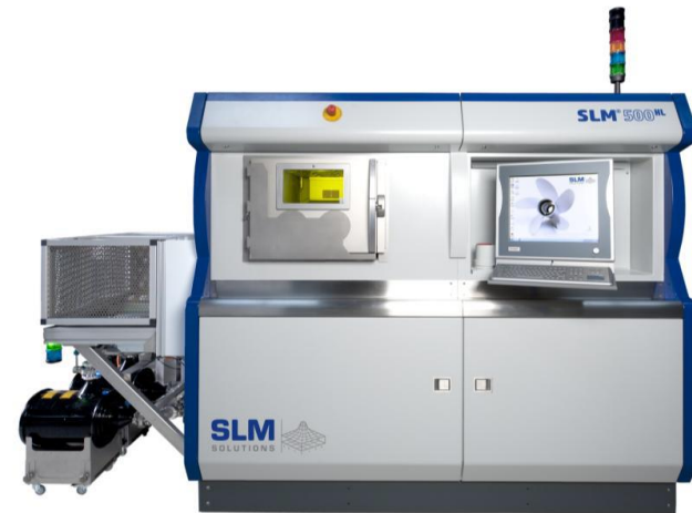
DST Group SLM Solutions SLM500 system - Dual 400 W fiber lasers
