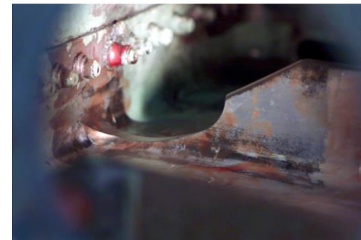
Optimised stiffener run-out
