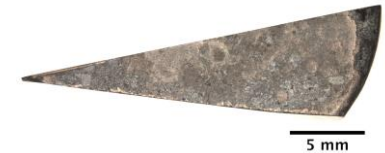
Thermal test specimen geometry – 20 degree wedge
