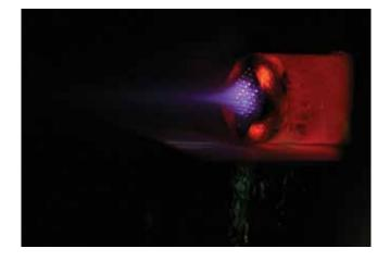
Alternatives such as electric propulsion have been in research and use for more than 50 years, with the traditional Gridded and Hall thrusters having been predominantly used. They have several disadvantages, such as the need for external neutralisation sources and accelerating grids, which demand high power and prevent their miniaturisation.
