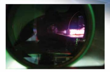
Intrinsic neutralisation of the propellant through charge exchange reactions is novel and gives the M-CXT a large advantage over conventional electric propulsion units which require additional and often bulky neutralisation units.
