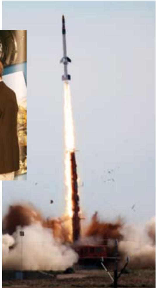
15 June 2006: Launch of the Hypersonic Collaborative Australia-US Experiment (HYCAUSE) which demonstrated ignition of a supersonic combustion ramjet (scramjet) engine at speeds close to Mach 10 during re-entry after climbing to an altitude of more than 450 km.
