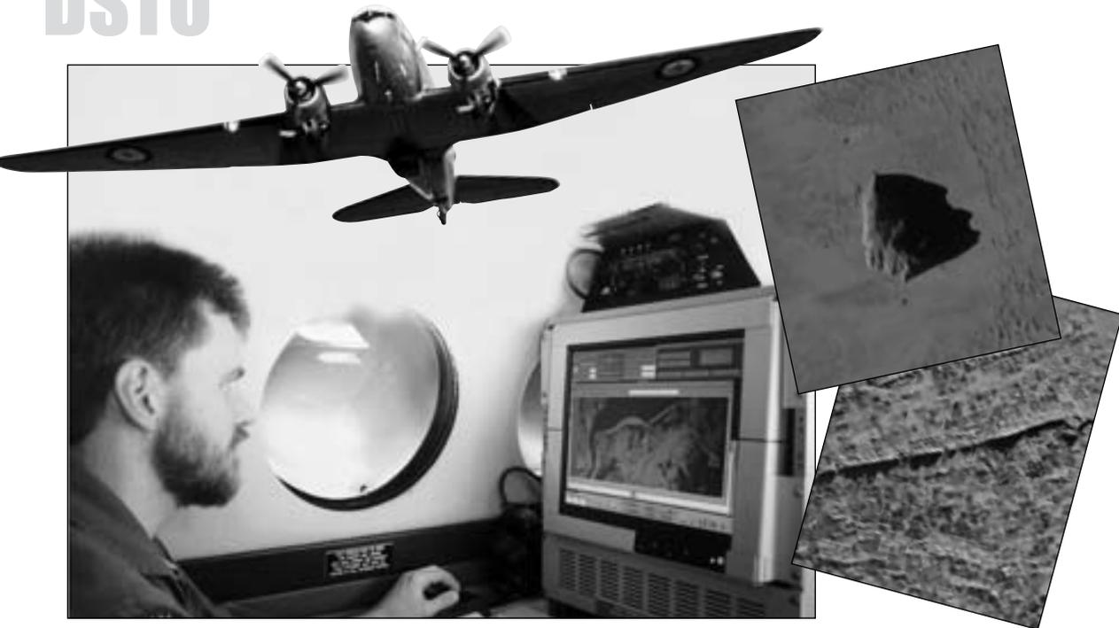
*The original C-47 AuSAR test bed. Nick Stacy operating the first Ingara real-time processor aboard the King Air 350 test bed, c. 1998. AuSAR images of Uluru and Saddleworth, Victoria.*
