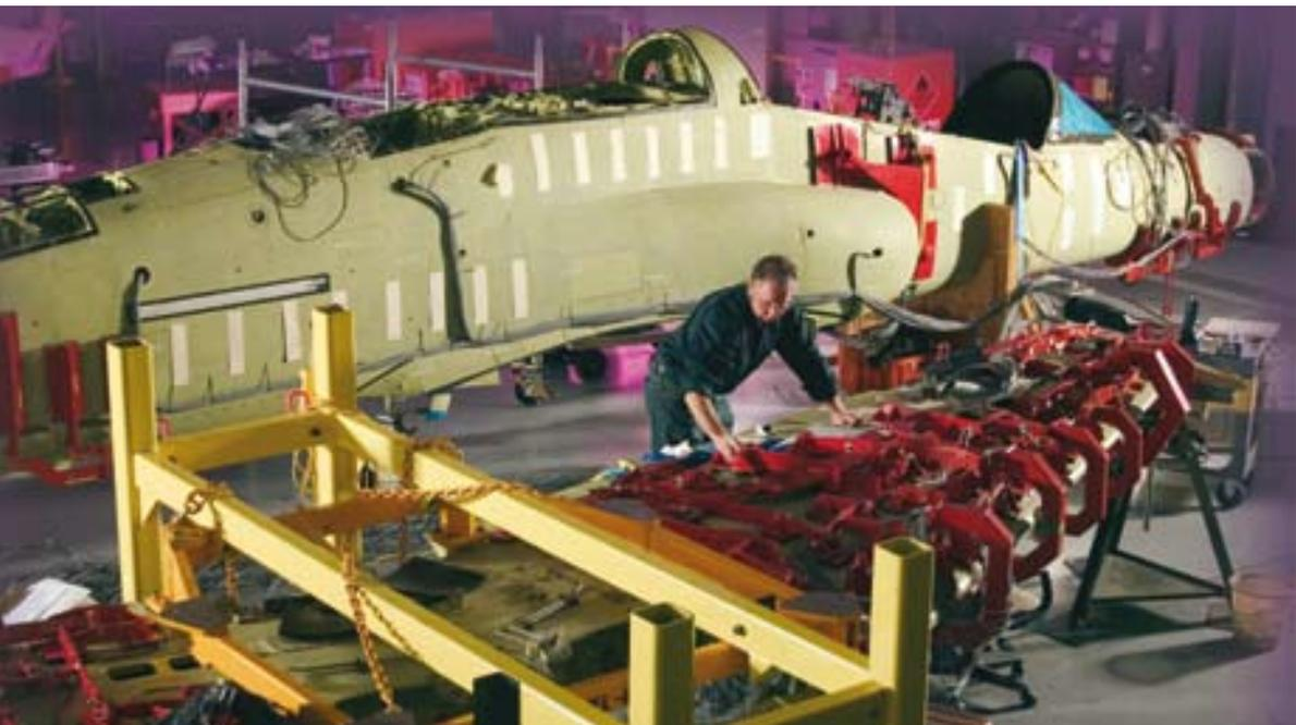
*Fatigue test of the Lead-in Fighter Hawk in the new H.A.Wills Structures & Materials Test Centre in Melbourne.*
