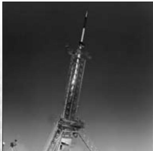
*Two-stage Skylark sounding rocket, Woomera. The Skylark launcher was built from Bailey bridge panels and shipped to Woomera in sections.*
