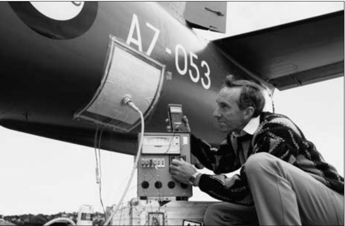
*Composite bonded repair patch being applied to a Macchi aircraft.*
