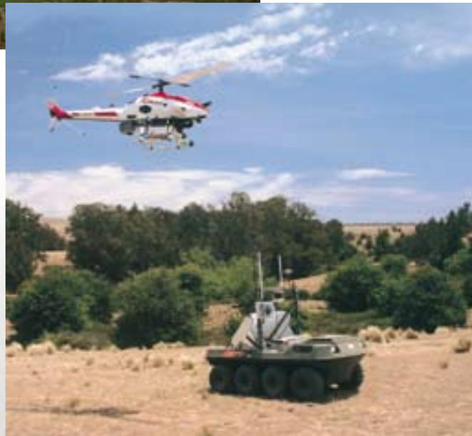
*Working with the universities of Sydney and Adelaide, DSTO demonstrated the ability of an unmanned ground vehicle to operate autonomously in difficult terrain by downloading maps from an unmanned aerial vehicle.*
