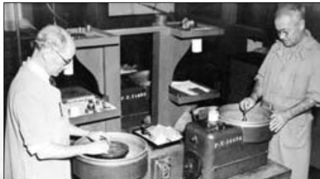
*Optical glass blanks being shaped for preparing lenses and prisms, c.1947.*
