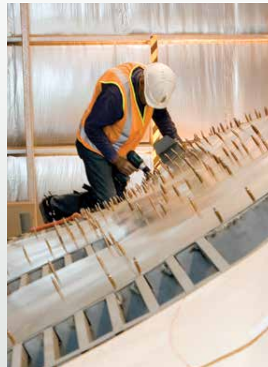
Above: The F-35 Joint Strike Fighter. Middle and Below: Iron Bird in final stages of construction, with close-up showing the arrays of stand-off spikes installed to facilitate measurement of the induced currents.
