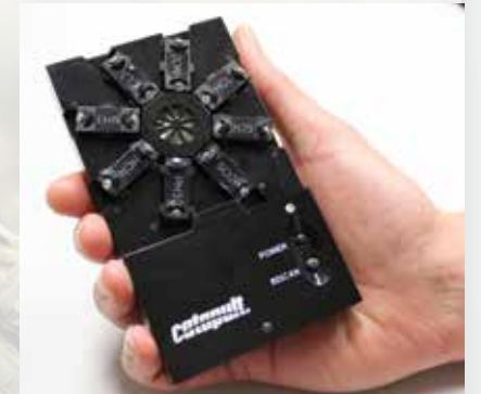
Black Canary – a wearable chemical detector.
