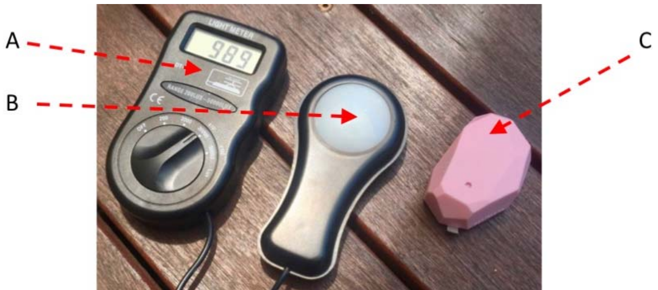
Figure 1 The experimental setup as used to collect 13 pairs of data points. (A) The Light Meter control unit, showing 9890 Lux; (B) the Light Meter light collecting dome, covering a light sensitive semiconductor device; (C) the Estimote Location Beacon, note the small (3 mm diameter) circular depression in the silicon housing covering the photosensitive diode embedded inside.
