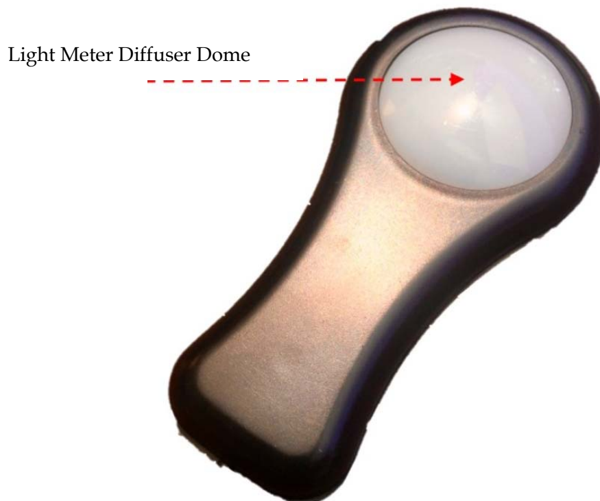
Figure 2 A close up view of the Light Meter collecting dome, measuring 40 mm diameter across the diffuser.
