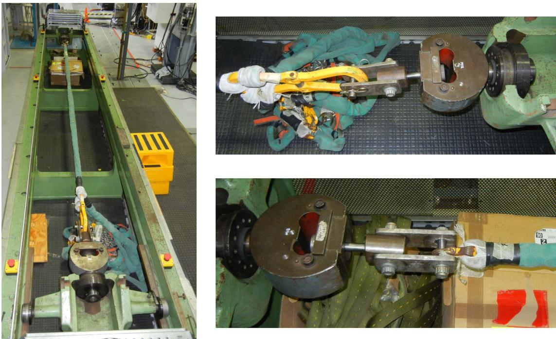
Figure 2: HUSLE installed in the Longbed Horizontal Tensile Testing Machine
