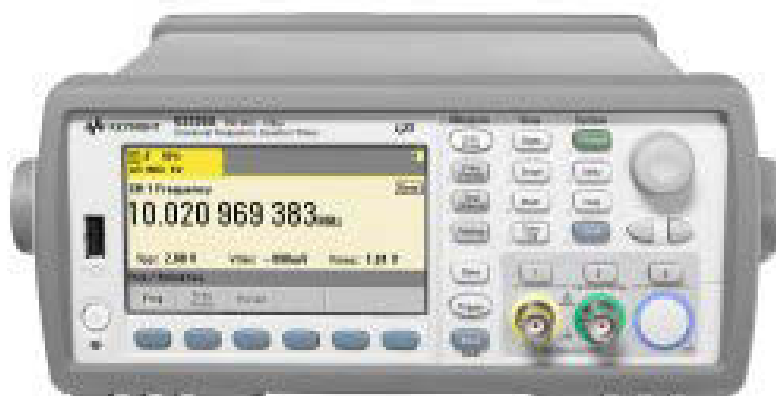
Figure 4: Keysight 53220A Universal Frequency counter (UFC)
