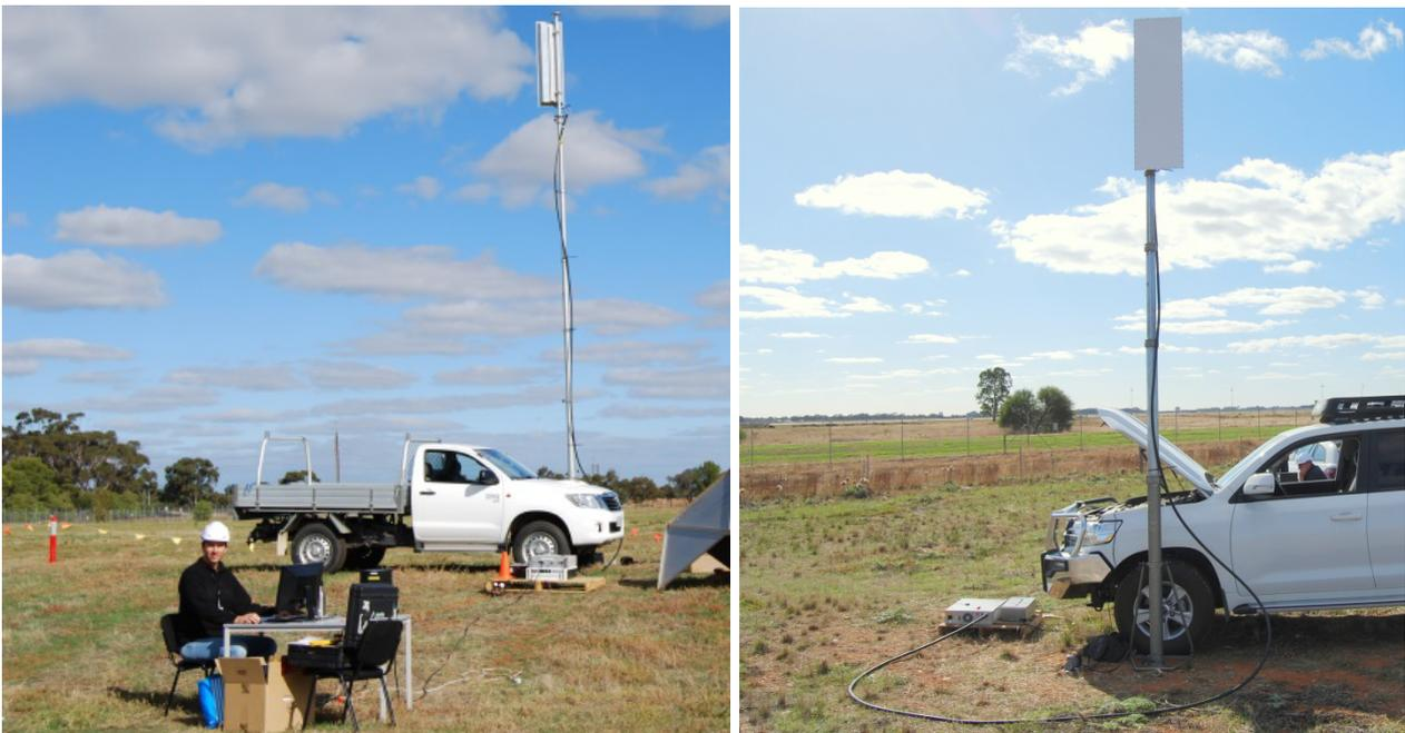
Figure 25. Monostatic RN1 deployment (left) and bistatic RN2 deployment (right) showing auxiliary equipment and masts
