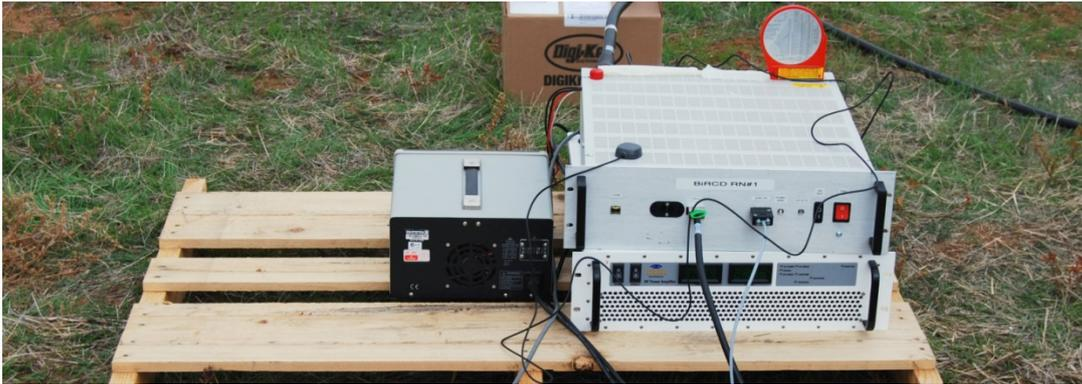
Figure 14. RNA (top-right) and PA (bottom-right) setup during the field trial
