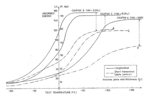
Figure 23: Longitudinal and short transverse Charpy curves for Vacumn Induction Melted (VIM) steel that is followed by either ESR (Coupons B and C) or Vacumn Arc Remelting (VAR) (Coupon A) (from [61]).
