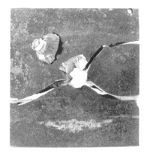
*Figure 14: Armour steel failure by a combination of shattering and discing. Note that the disc is associated with a partially-formed plug (from [29]).*
