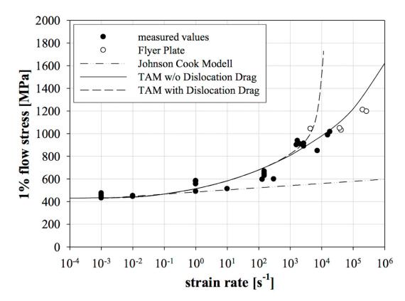
*Figure 10: Compressive true flow stress at 1% true plastic strain for 1045 steel at strain rates from 10-3 to 105 s-1, compared to the Thermal Activation Model (TAM), TAM with Dislocation Drag and the Johnson Cook Model (from [21]).*
