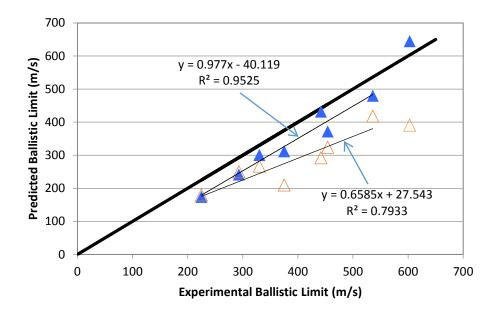
Figure 7: Experimental vs predicted ballistic limits from ductile hole formation theory, Eqn 1, for two quasi-static measures of true compressive strength,  $\sigma_0$  (closed symbols) and  $\sigma_y$ (open symbols) [3]. Linear regression lines are plotted through all data except for the data point with abnormally high work hardening.
