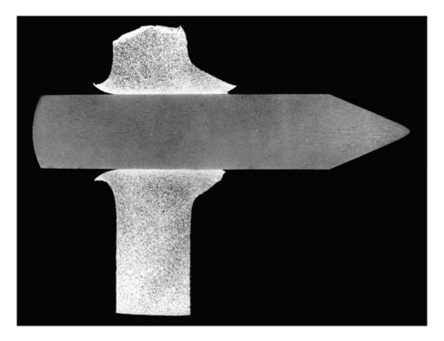
*Figure 1: Example of a mild steel plate perforated by a conical, non-deforming projectile, illustrating the ductile hole formation failure mechanism (from [3]).*
