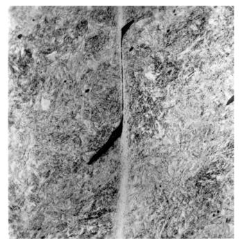
*Figure 17: Adiabatic shear band (central white band from top to bottom of image). Significant shear strains are evident from the displacement of the dark inclusion by the shear band (from [14]).*
