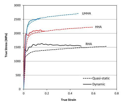
*Figure 9:* Compressive true stress – strain curves for MARS armour steels, MARS 190 (RHA), MARS240 (HHA) and MARS300 (UHHA) with dynamic strain rates of 4800s<sup>-1</sup>, 3800s<sup>-1</sup> and 1500-2500s<sup>-1</sup>, respectively (from [22]).
