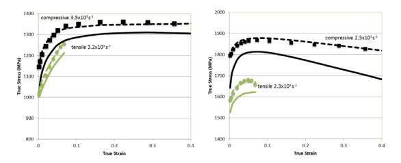
Figure 12: Compressive and tensile flow stresses for two quenched and tempered steels at nominal identical strain rates: left, 290HV30 (tensile 3.2x10<sup>3</sup> s<sup>-1</sup> and compressive 3.5x10<sup>3</sup> s<sup>-1</sup>) and right, 410HV30 (tensile 2.3x10<sup>3</sup> s<sup>-1</sup> and compressive 2.5x10<sup>3</sup> s<sup>-1</sup>) (after [27]). Associated Zerilli-Armstrong, -----, and Johnson-Cook, -----, predictions are also shown.
