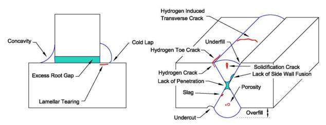
*Figure 19: Schematic of weld defects and discontinuities [51]. Cracks are depicted in red and gaps between materials are depicted in green.*
