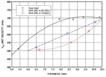
*Figure 21: The* V<sub>50</sub> *ballistic limit for Bulgarian dual hardness armour, HHA and RHA against* 0.30 Cal APM2 at 0° obliquity (after [57]).
