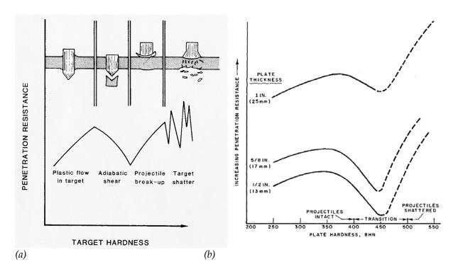
*Figure 2:* The relationship between the hardness of a monolithic armour steel plate and its performance against armour piercing projectiles. Changes in failure mechanisms result in a complex, discontinuous relationship between plate hardness and penetration resistance, expressed schematically (left, from [5]) and in terms of Brinell hardness values (right, from [1]) for an unspecified armour piercing projectile.
