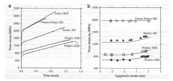
Dynamic tensile properties have also been measured. Figure 11 compares quasi-static tensile and dynamic tensile properties for a range of quenched and tempered steels.
