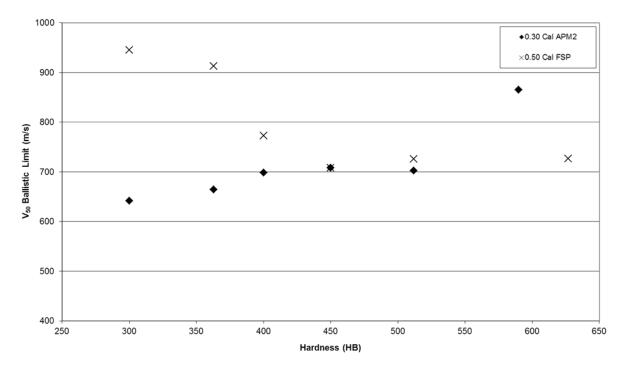
*Figure 3:* Influence of increase in hardness on the  $V_{50}$  ballistic limit for 10 mm Bisalloy armour steel plates against 0.30 Cal APM2 and 0.50 Cal FSPs (after [8,9]).
