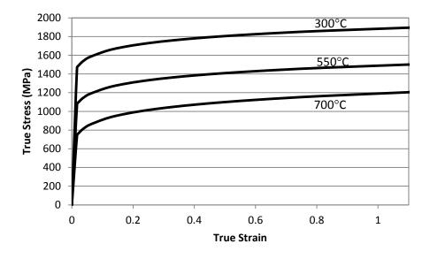
*Figure 6:* Compressive quasi-static true stress – strain curves for a 4130 steel that has been quenched and tempered at 300 °C (480HV), 550 °C (370HV) and 700 °C (260HV) with flow stresses described by  $\sigma = \sigma_0 \varepsilon^n$  [19].
