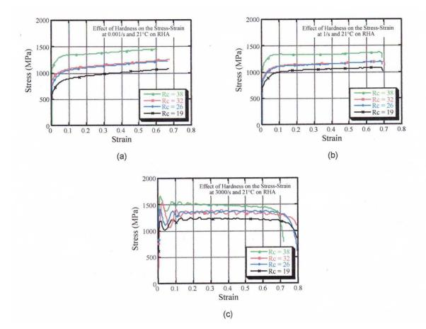
Figure 13: Compressive stress – strain curves at different surface hardnesses (HRc 38 ≅ 353HB, HRc 32 ≅ 301HB, HRc 26 ≅ 258HB and HRc 19 ≅ 223HB) for RHA at strain rates of: (a) 0.001 s<sup>-1</sup>; (b) 1s<sup>-1</sup>; and (c) 3000s<sup>-1</sup>. (from [28]).
