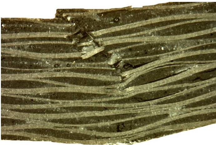
Figure 23 - Example specimen failure for four-point bend loading. A silicon sheet is used to disperse the applied load underneath either loading nose.
