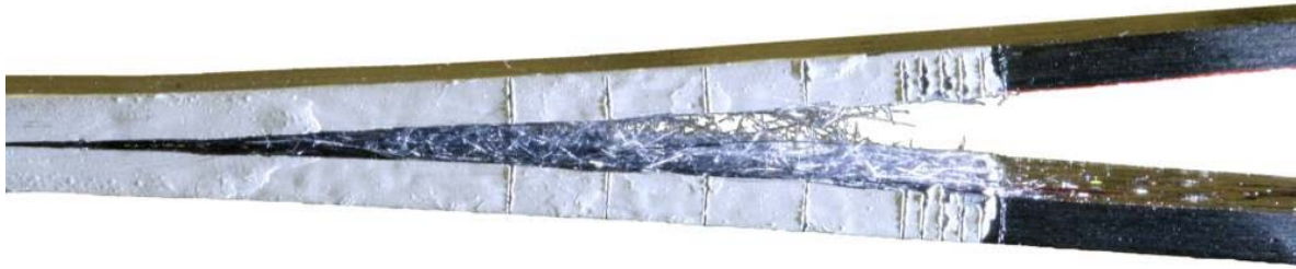
Figure 28 – Example of fibre bridging occurring along the crack front of a K3600 + E21 DCB specimen.
