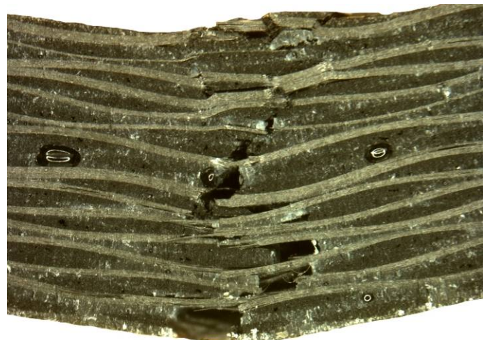
Figure 24 - Micrographs showing (i) compressive failure due to bearing on the top face of the specimen, and (ii) tensile dominated failure on the bottom of the specimen, which is the desired failure mode for the four point bend test.
