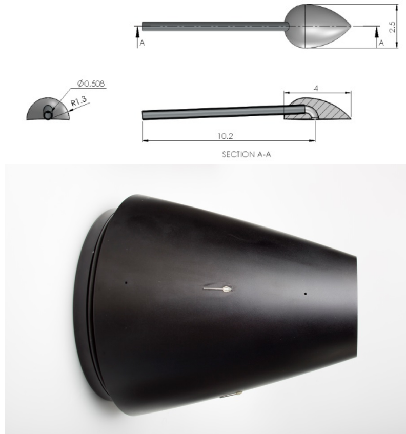
Figure 5: Preston tube and fairing (top, dimension in mm) and Preston tubes in place on a tail cone segment (bottom).
