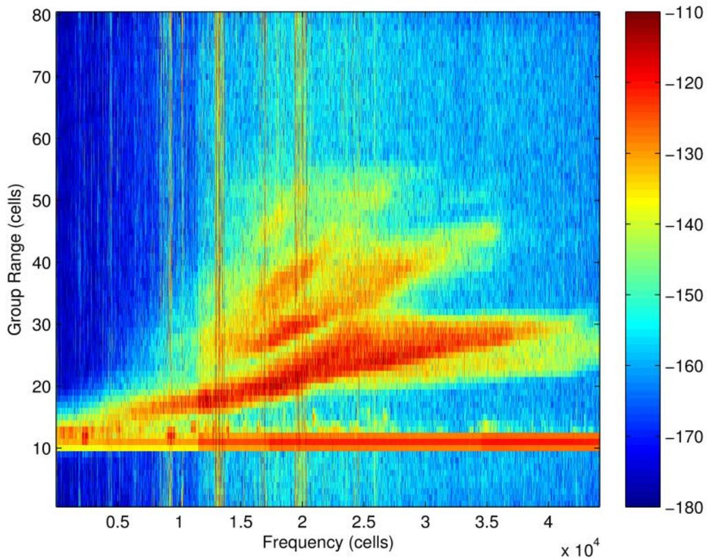
Figure 6. The 192 overlapped time series per 100 kHz yield an ionogram with very high frequency resolution
