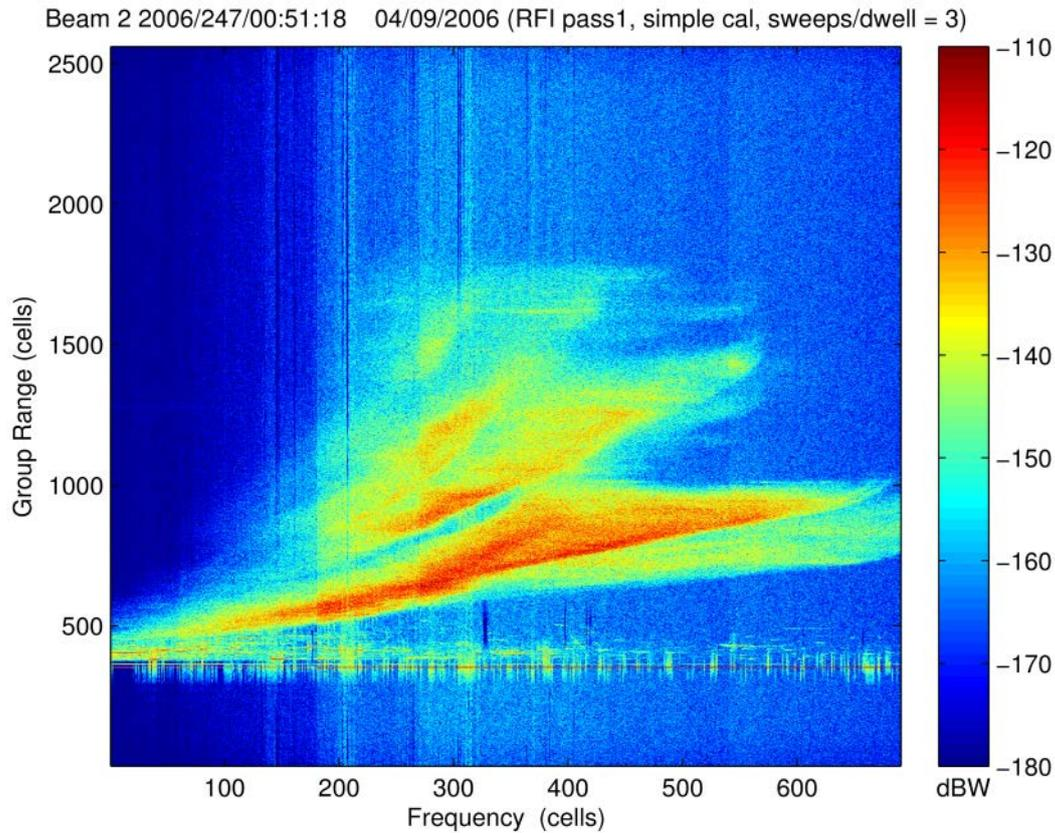
Figure 12. BSI after first pass of the RFI clean-up algorithm reprocessed to 2560 range cells and 3 frequency cells per 100 kHz to give 690 frequency cells across the 5-28 MHz band
