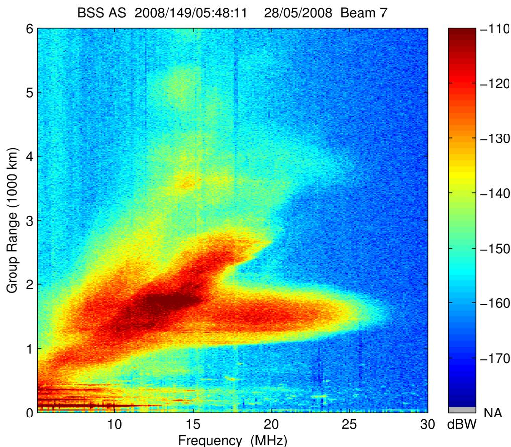
Figure 27. High resolution backscatter ionogram with pixel resolution 6.1 km by 100 kHz showing *E<sub>s</sub>* both from backscatter at 1000-2000 km and from multi-hop QVI at close range. Also visible is the ground wave return at 50 km. The calibration signal is just off the bottom of the image at -24.4 km.
