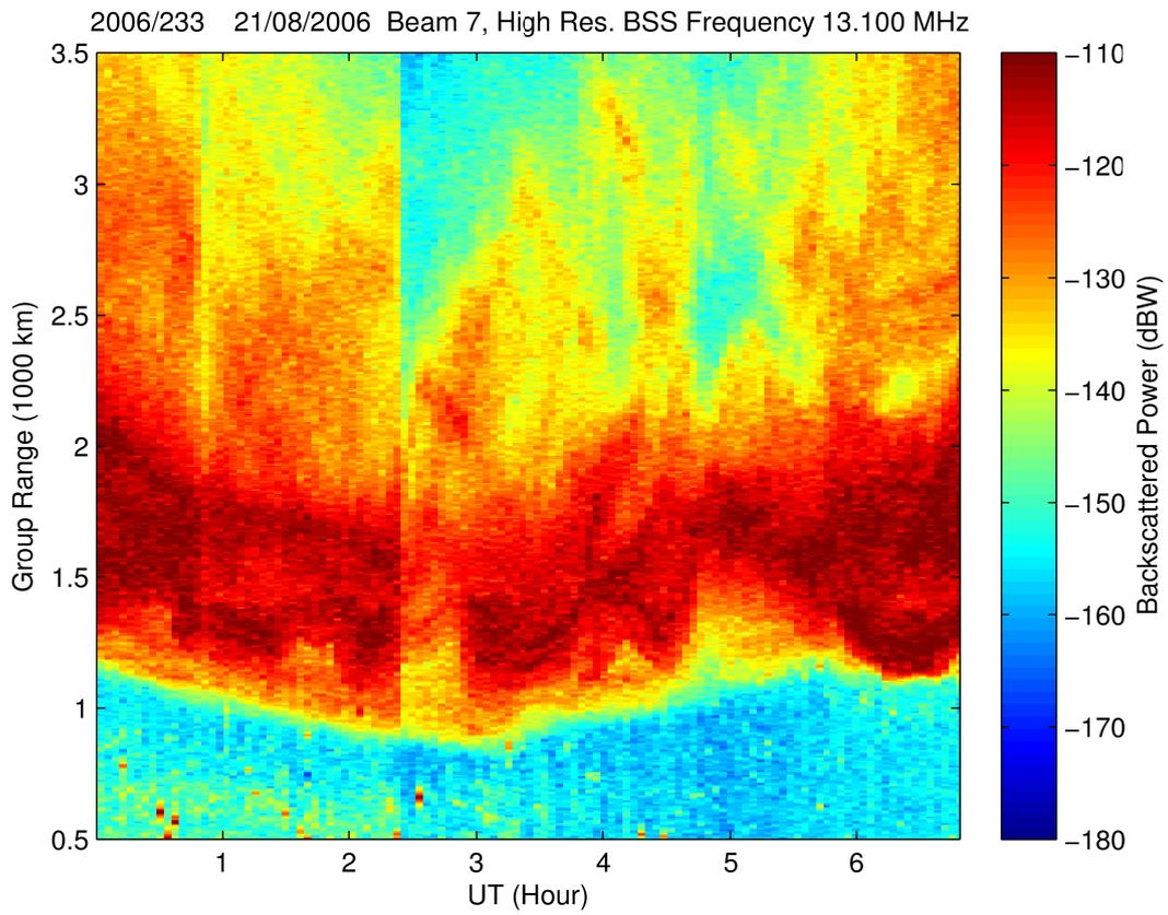
Figure 33. Backscattered power obtained from high resolution processing to resolution 6.1 km by 200 kHz showing the greater detail visible on comparison with the standard processing of Figure 32.
