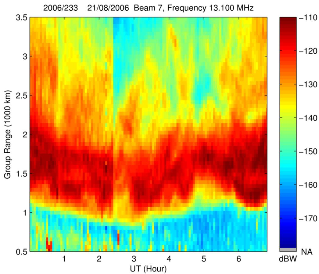
Figure 32. Backscattered power obtained from standard BSS processing at resolution 48.8 km by 200 kHz for comparison with Figure 33.
