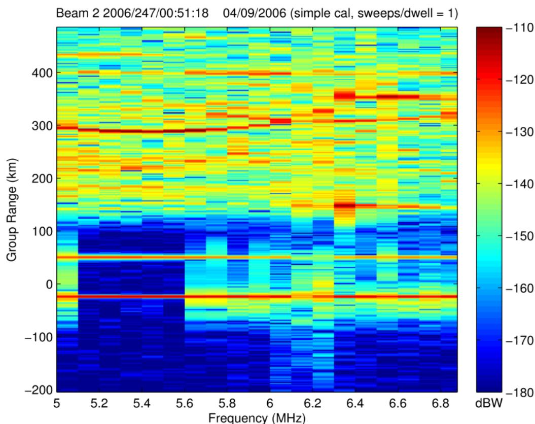
Figure 21. Highest range resolution BSI (2 km by 100 kHz) zoomed to show the calibration signal at -24.4 km, the ground wave at 49.9 km and quasi-vertical incidence F2 O and X traces at approximately 300 km (in amongst other signals).
