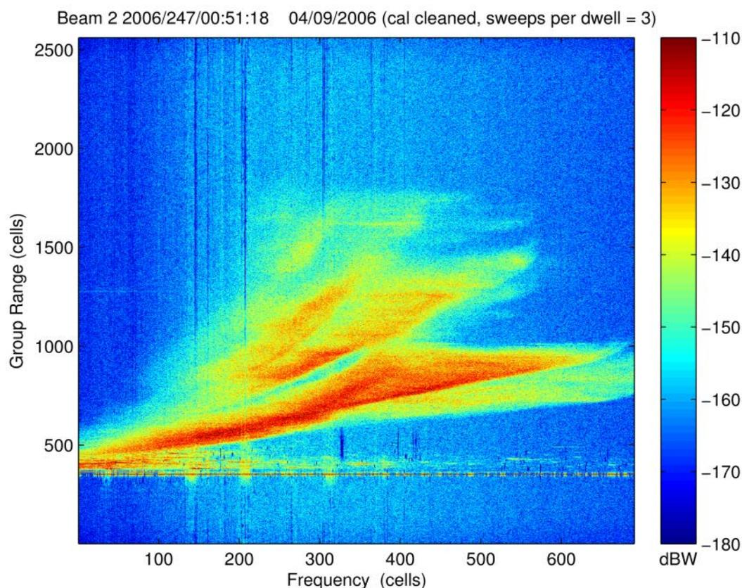
Figure 24. Final RFI cleaned and calibrated backscatter ionogram at a resolution of 6.1 km by 3 frequencies per 100 kHz (based on the same data as the standard image presented in Figure 2).
