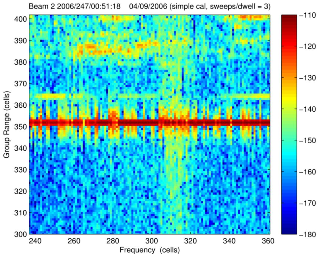
Figure 20. After the second pass of the RFI removal algorithm, on comparison with Figure 19, the residual RFI extending away from the calibration signal has been reduced, but the integrity of the calibration signal has been adversely affected and there are more artefacts close to the calibration signal
