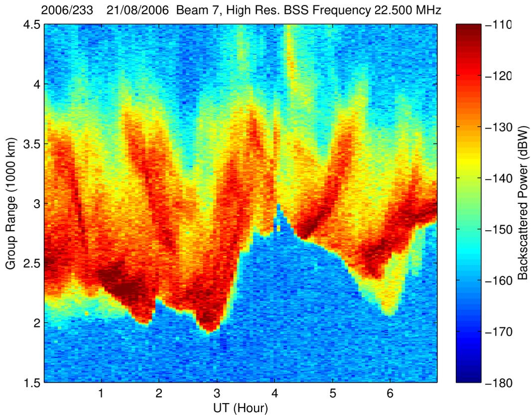
Figure 34. At 22.5 MHz most of the propagation shown here is beyond the E horizon. Visible in this image are regions of focussed power at longer ranges than the leading edge. The high resolution processing (at 6.1 km by 100 kHz) shows the detail of the progression of the regions of focus with time.
