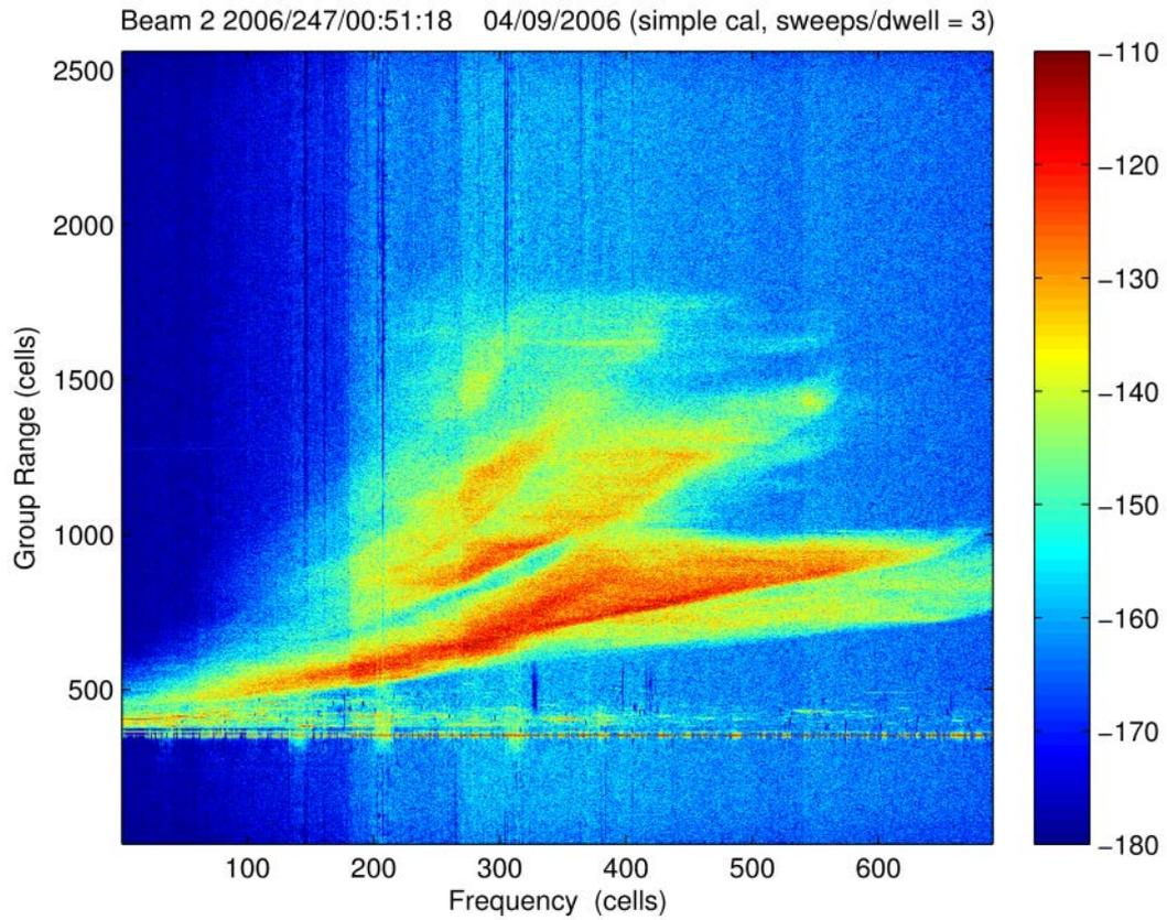
Figure 18. Backscatter ionogram after the second pass of the RFI removal algorithm but with only simple calibration at this stage. On comparison with Figure 12 it can be seen that the feathery remains of RFI attached to the calibration signal have been reduced.
