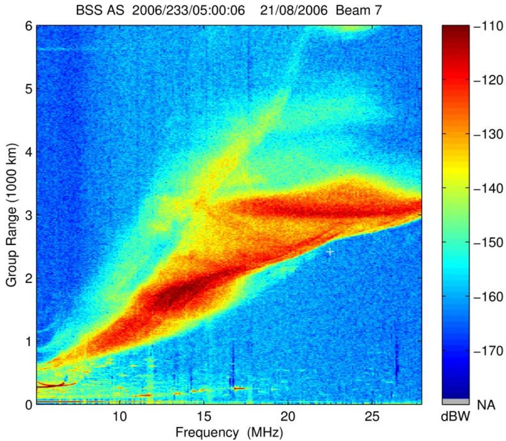
Figure 35. At 22.5 MHz there is a region of focussed power at approximately 3000 km, a few hundred km beyond the LE at approximately 2700 km. Also visible are QVI F2 O and X traces, possibly the 2 hop QVI traces, the ground wave at 50 km, an Es LE out to about 2000 km, and O-X splitting of the F2 LE. The resolution of the image is 6.1 km by 100 kHz.
