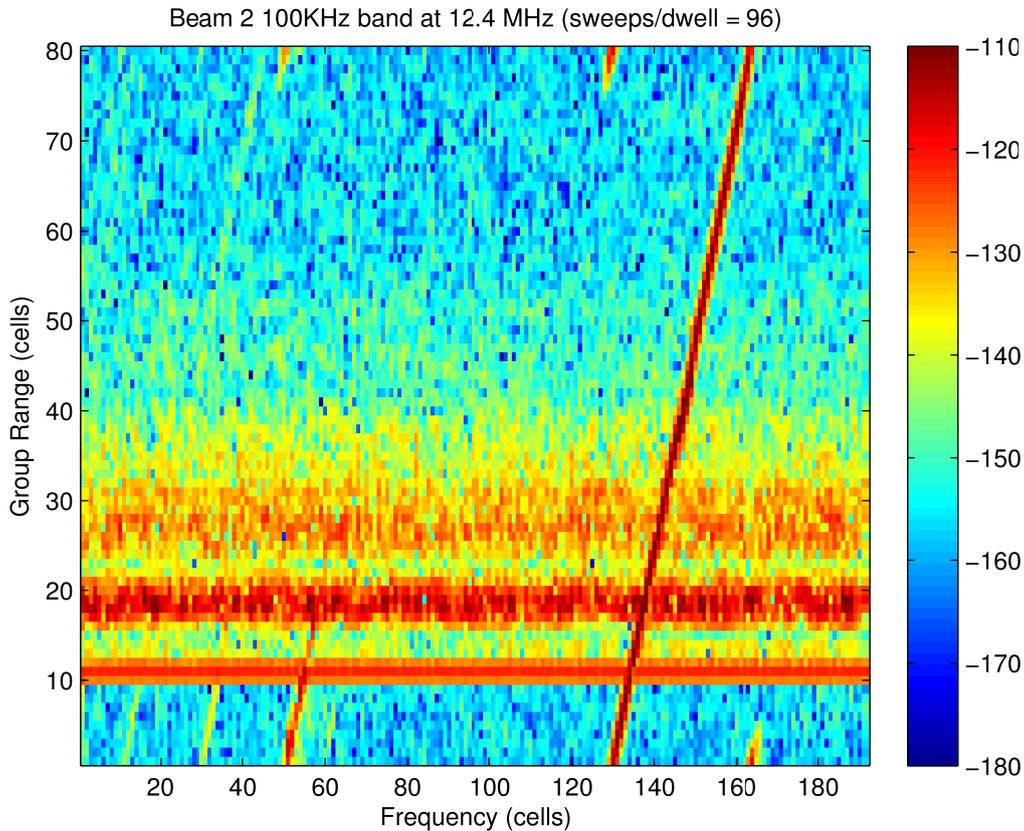
Figure 7. The 192 spectra for one dwell starting at 12.4 MHz. The resolution is approximately 195 km by 384 Hz. The calibration signal is visible at range cell 11. The diagonal lines are narrow band RFI, transmitted at fixed frequencies but have slopes here corresponding to the sweep rate of the BSS.
