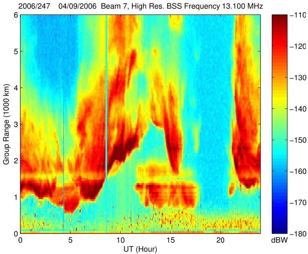
Figure 29. Backscattered power as a function of group range at 13.1 MHz for a 24 hour period using high resolution processing and incoherent averaging to the standard resolution of 48.8 km by 200 kHz. Even though the resolution is the same as for the standard processing used for Figure 28, the image appears crisper, the edge of the backscattered power is cleaner and the meteor echoes are visibly less spread in the range dimension, being confined to one or two range cells.
