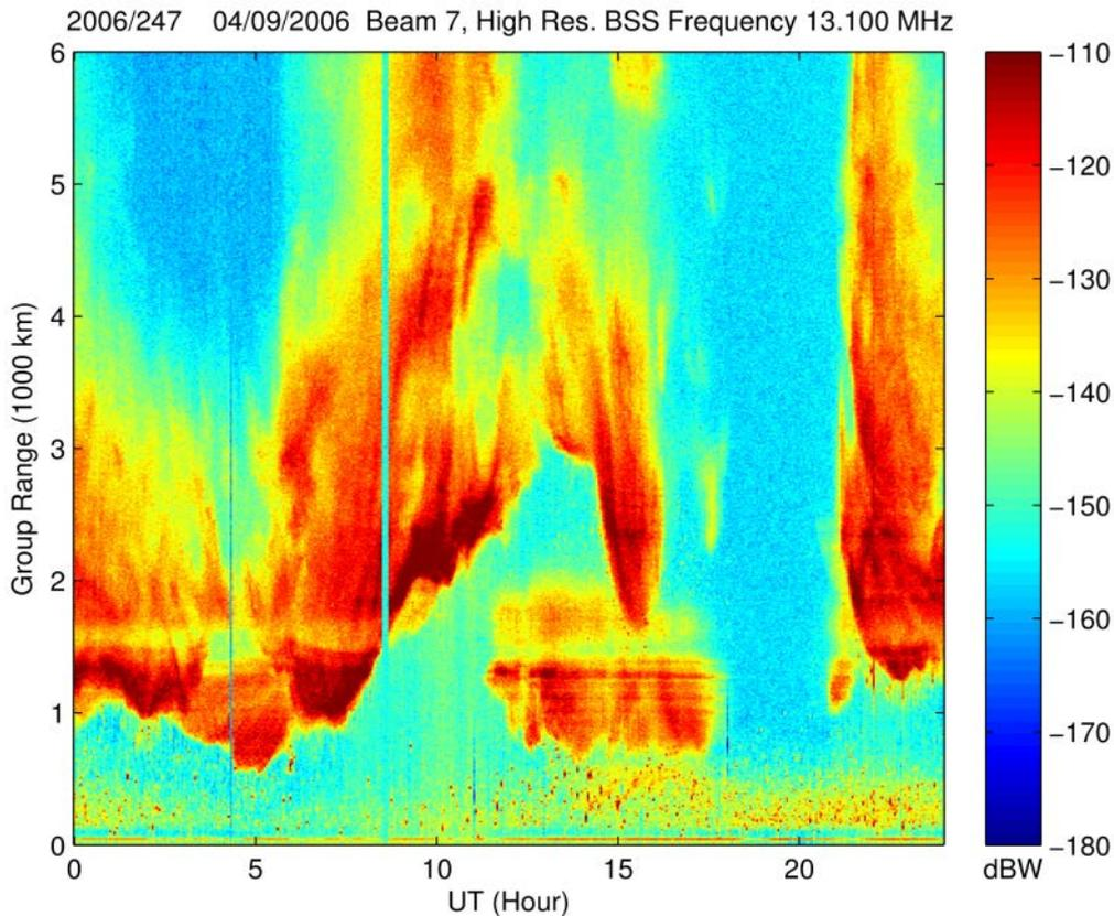
Figure 31. Incoherently averaging the power over 6 frequency samples to resolution 6.1 km by 200 kHz reduces both the noise and backscattered power variance, as expected, without an obvious loss of clarity. In fact the higher power backscatter just inside the leading edge is better defined, for example, at around 0630 UT.
