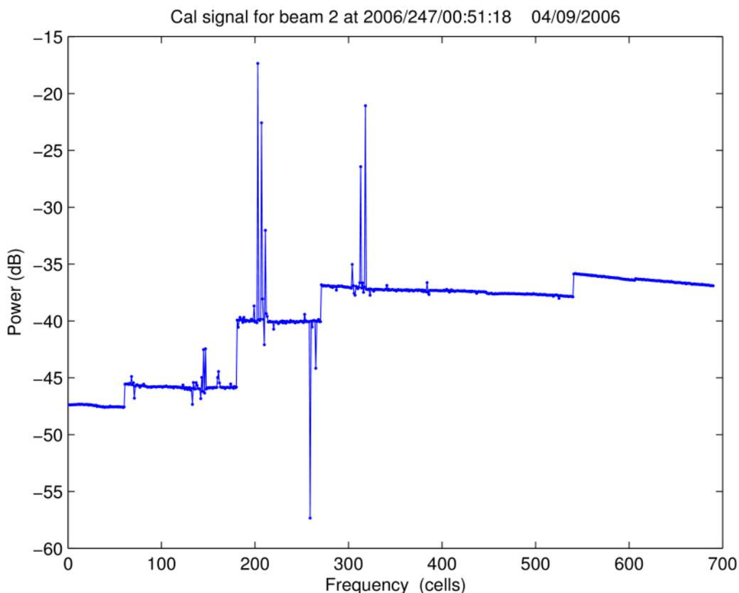
Figure 22. RFI is frequently strong enough to contaminate the calibration signal.
