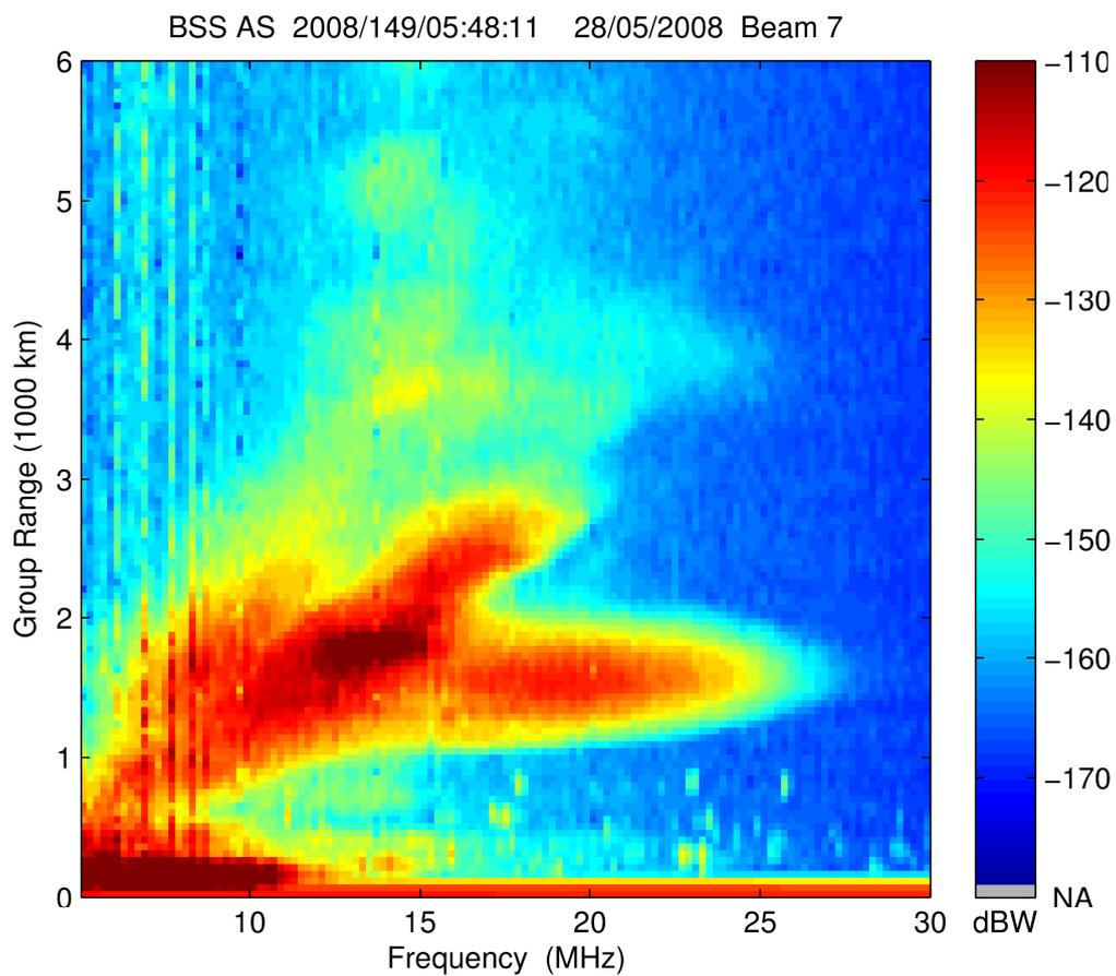
Figure 26. Standard backscatter ionogram with resolution 48.8 km by 200 kHz showing Es propagation from ranges 1000 to 2000 km. At close range, 100 to 300 km just beyond the calibration signal, there are unresolved quasi-vertical incidence traces.
