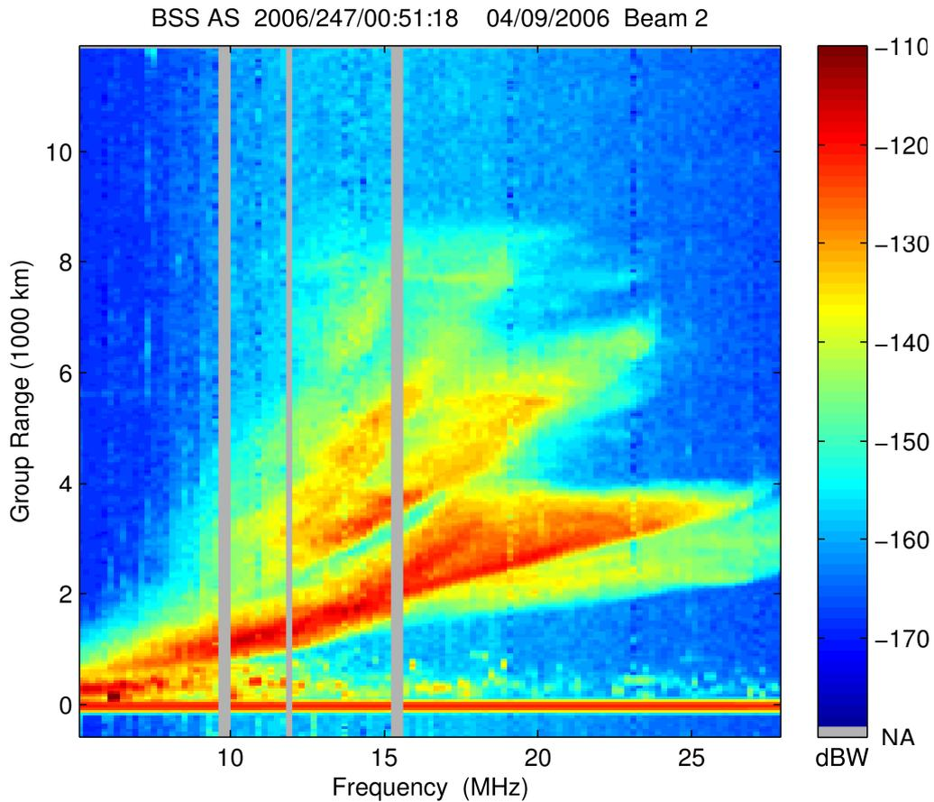
Figure 2. Standard processing removes RFI by excluding contaminated spectra from 48 in a 200 kHz band and taking the average of the remainder. If the number of remaining spectra is less than 6 all the data is excluded (grey vertical bands) and interpolation from neighbouring good frequencies is subsequently performed (not done in this figure). The standard resolution is 200 kHz by 48.8 km.
