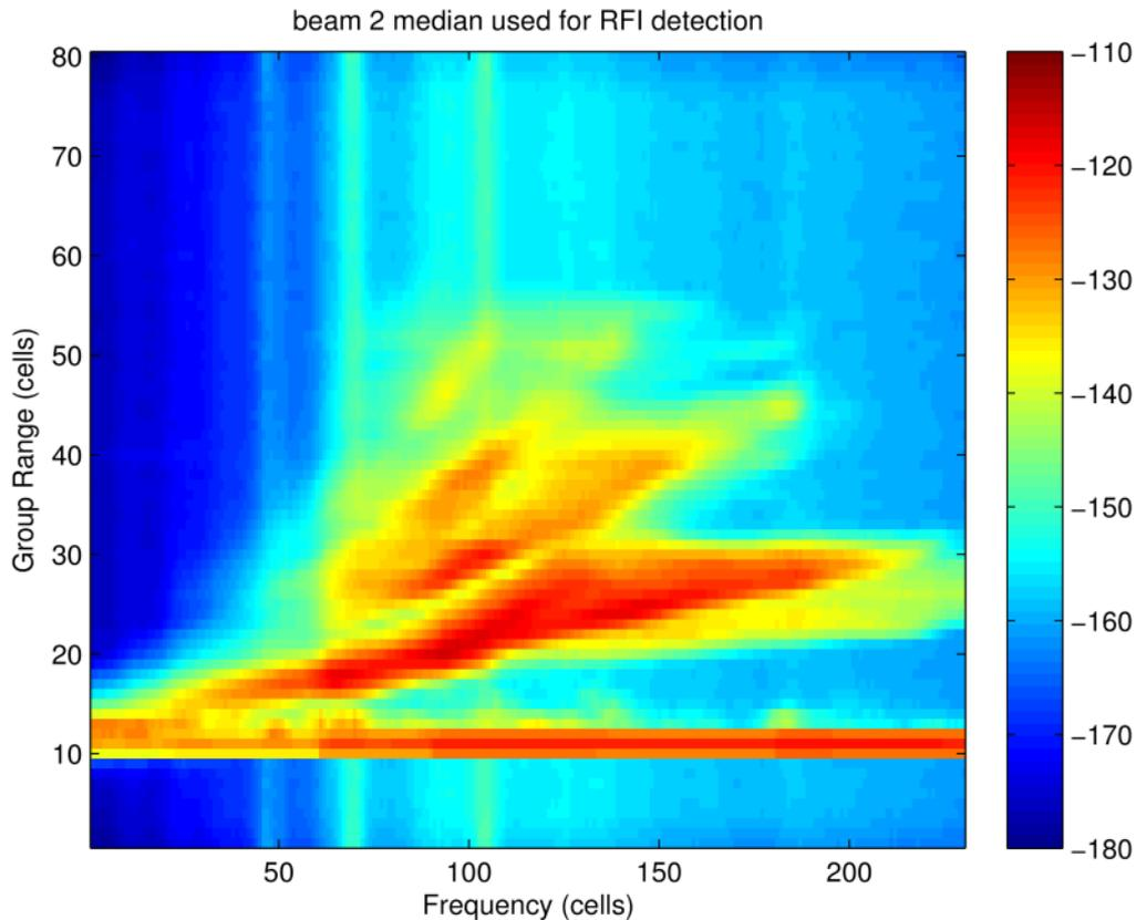
Figure 8. Median ionogram used for RFI detection. The resolution of this ionogram is 195 km by 100 kHz. Some residual RFI is visible.
