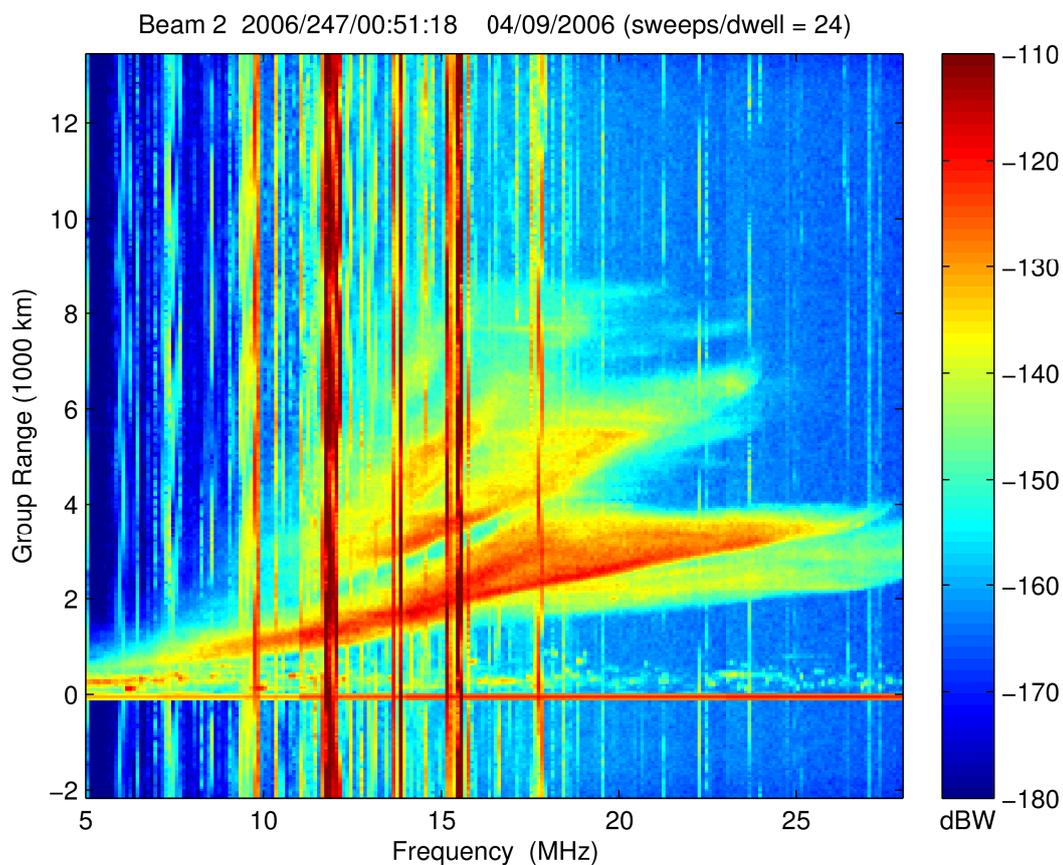
Figure 1. Backscatter ionogram created using the standard processing without RFI rejection. The vertical lines are the unwanted RFI signals contaminating the data. The horizontal line at -24.4 km is the injected calibration signal. The other main sources of power are the desired backscattered signal and potentially azimuthal side-lobe power.
