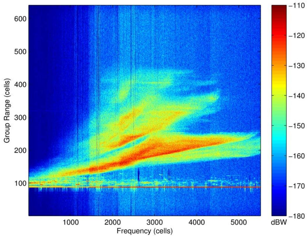
Figure 13. The first pass BSI reprocessed to 640 range cells and 24 frequency cells per 100 kHz for the second pass. Residual RFI remaining after the first pass of RFI mitigation algorithm appears as "feathering" on large signals such as the calibration signal
