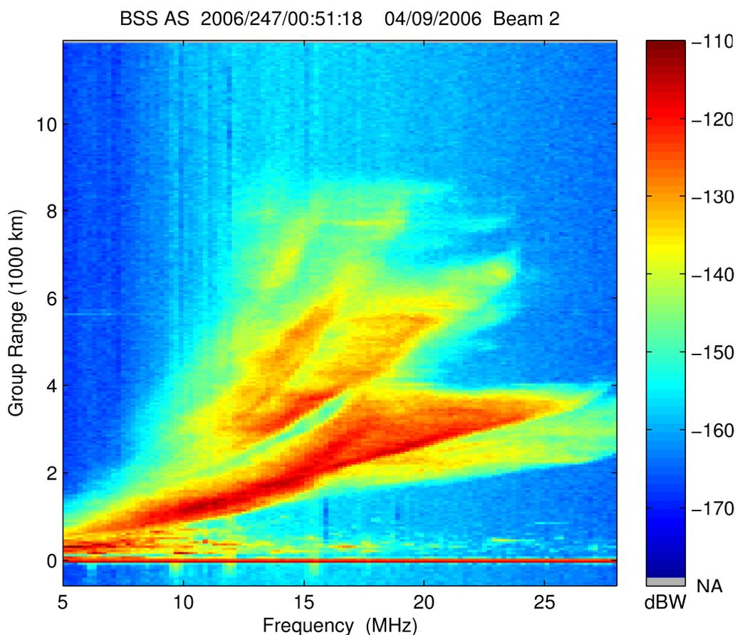
Figure 25. High resolution backscatter ionogram processed to have the standard resolution of 48.8 km by 200 kHz. Note the substantially cleaner appearance on comparison with Figure 2.
