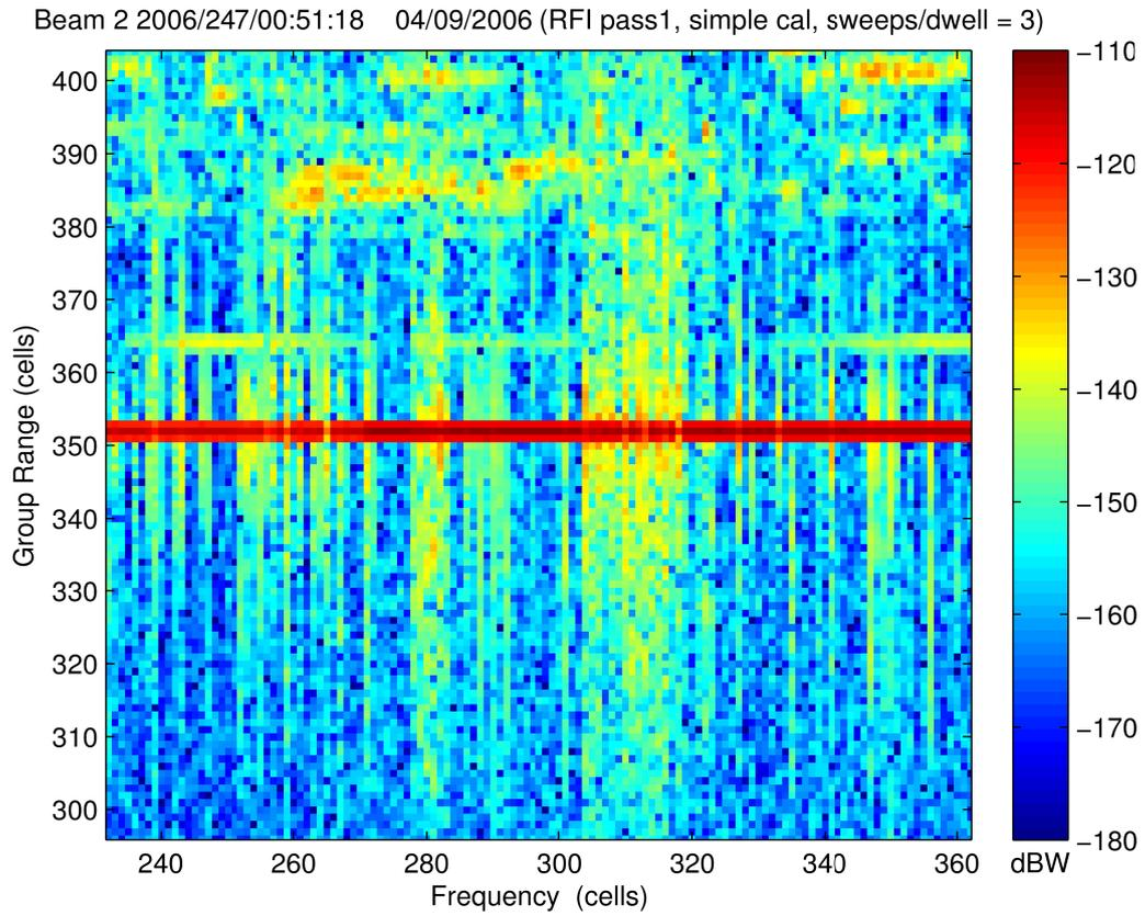
Figure 19. Zoomed BSI after the first pass of the RFI removal algorithm showing detail around the calibration signal for comparison with Figure 20
