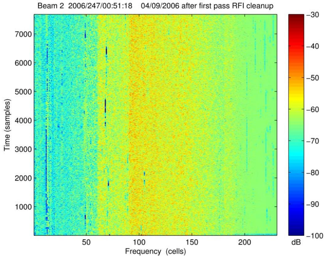
Figure 11. Received power in the time domain after first pass RFI removal
