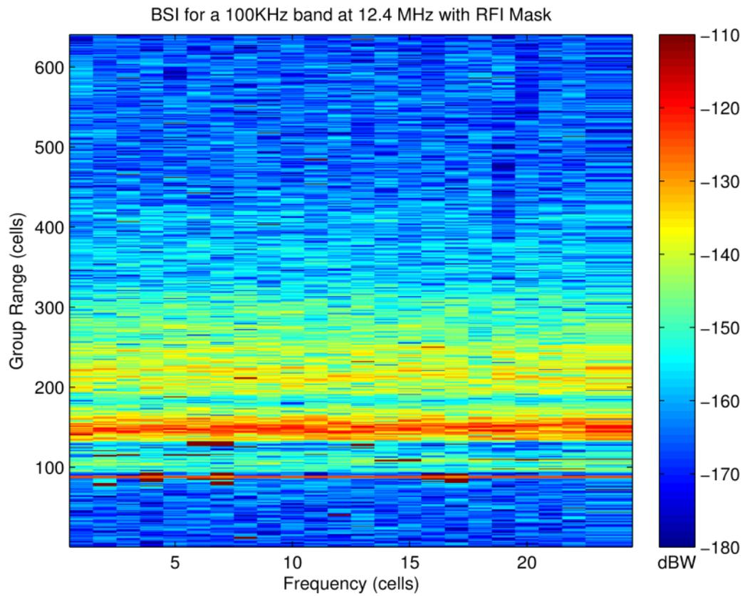
Figure 15. BSI at 12.4 MHz, processed for second pass RFI removal. The data to be removed is coloured dark red, the colour of the maximum display power.
