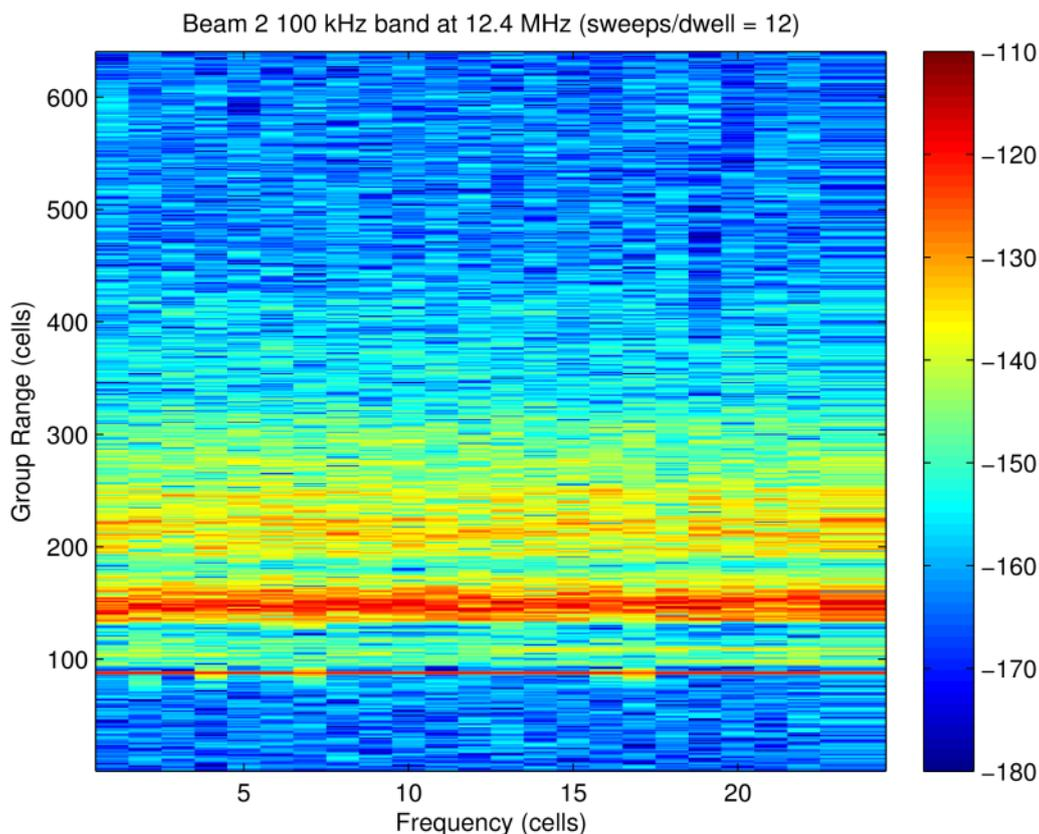
Figure 14. BSI at 12.4 MHz after processing to 640 range cells and 24 frequency cells per 100 kHz. Residual RFI remaining after the first pass of RFI mitigation algorithm appears as “feathering” and can be seen here attached to the calibration signal in frequency cells 4, 7 and 17
