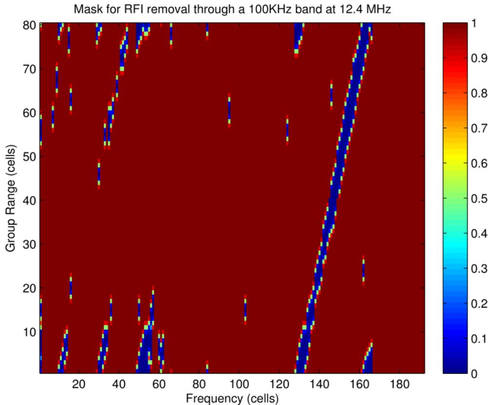
Figure 10. The tapered notches created for RFI excision corresponding to Figure 9
