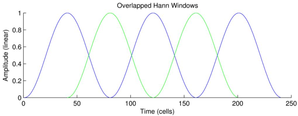
Figure 5. A 240 sample time series multiplied by overlapped Hann (sine squared) windows would produce 5 segments of 80 samples for spectral analysis. At each time cell the original signal is the sum of the 2 overlapped components
