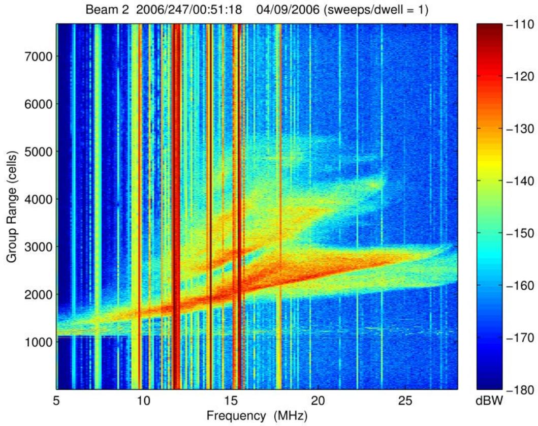
Figure 3. BSS data processed for maximum range resolution (2 km) with 7680 range cells by 230 frequency cells. Significant RFI is evident
