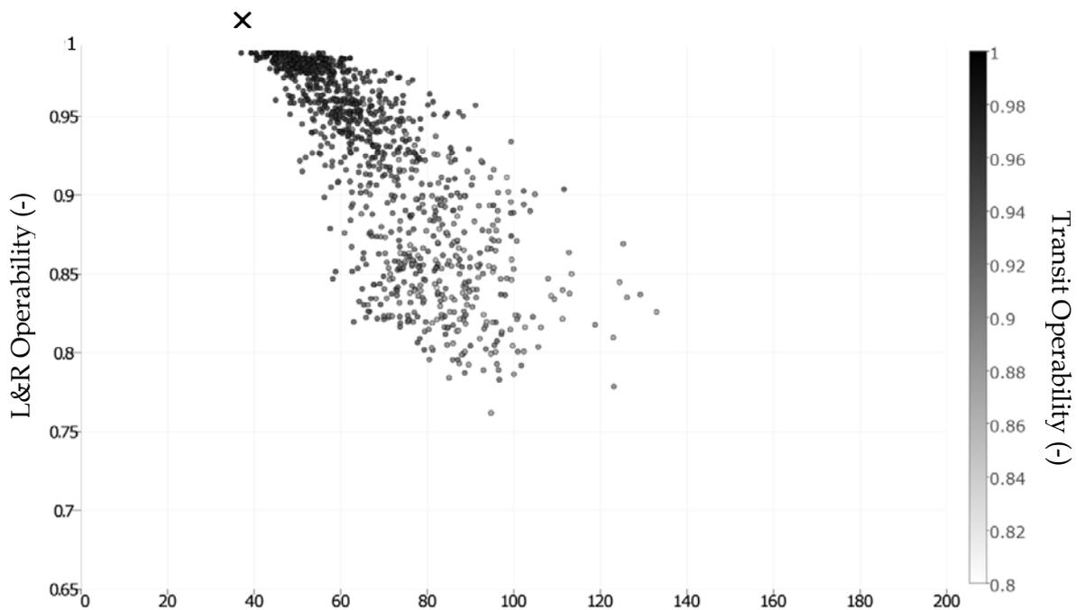
Figure 6. Scatter plot of the offshore patrol vessel type hullform design space in SS3 illustrating the relationship between L&R operability and Total Resistance per tonne Displacement at 14 knots. Colour gradient represents the respective Transit operability.
