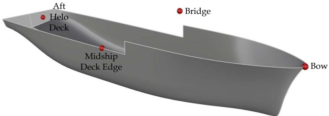
Figure B3 Representation of the four locations used for assessing the seakeeping operability indices
