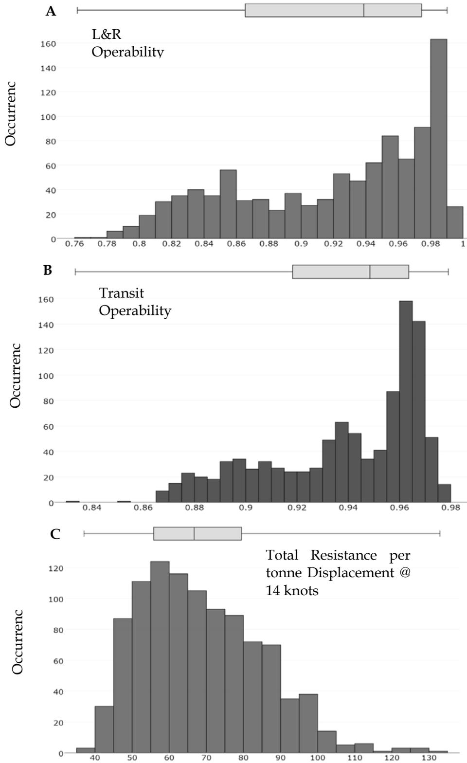
Figure 7. Histogram plots of the offshore patrol vessel type hullform in SS3 for: (A) L&R operability; (B) Transit Operability; (C) Total Resistance per tonne Displacement at 14 knots
