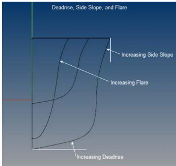
Figure A7. Body Plan view detailing the following hull design variables: Deadrise Aft, Mid and Fwd; Side Slope Aft, Mid and Fwd; Flare Aft, Mid and Fwd
