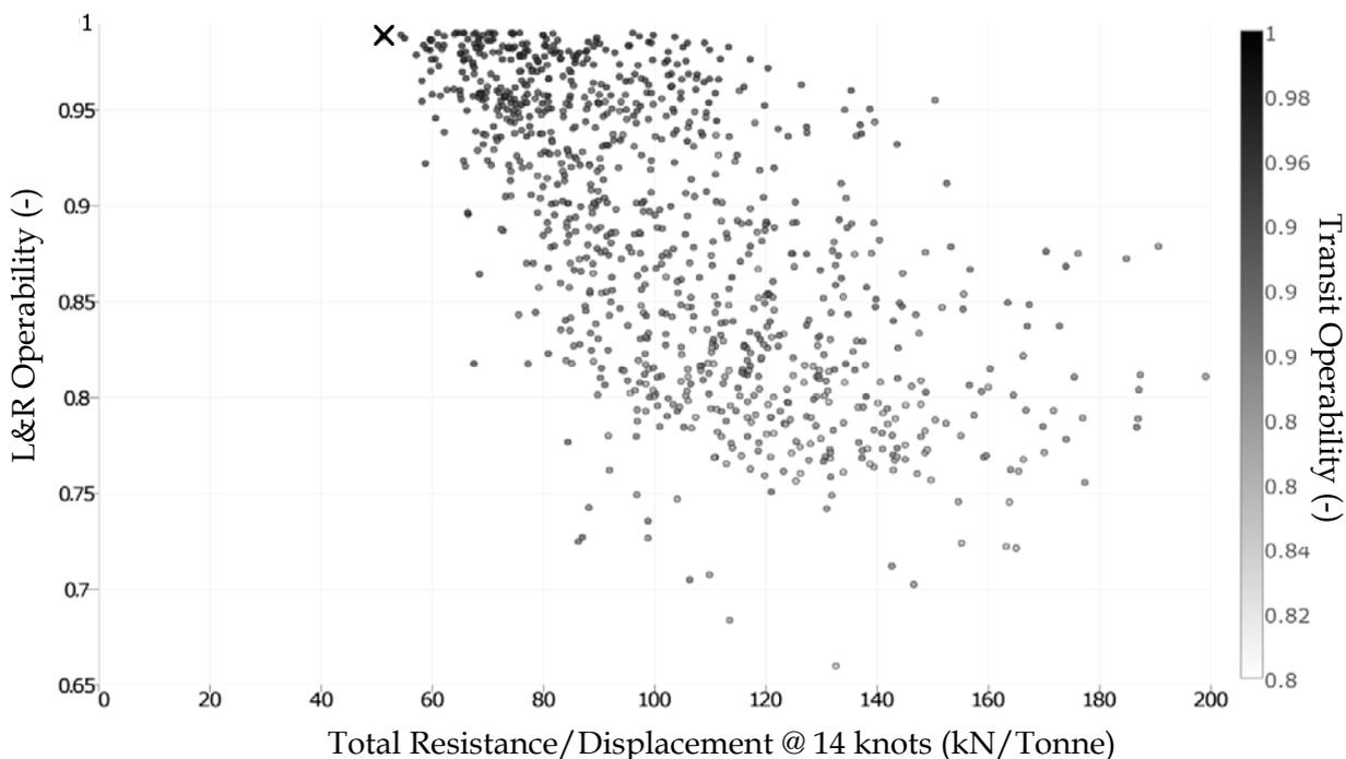
Figure 8. Scatter plot of the frigate type hullform design space in SS3 illustrating the relationship between L&R operability and Total Resistance per tonne Displacement at 14 knots. Colour gradient represents the respective Transit operability.
