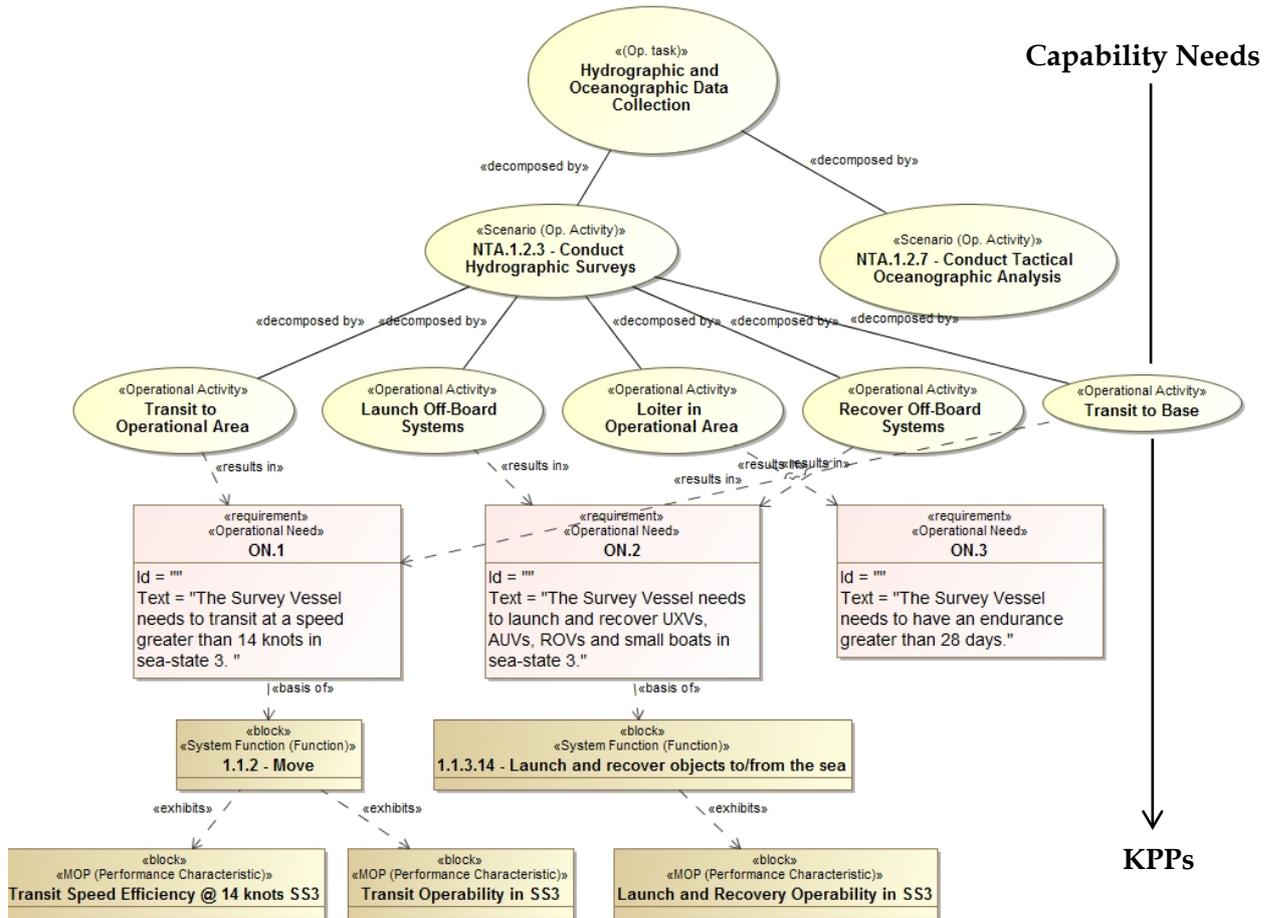
Figure 3. Functional breakdown diagram describing the traceability process between the KPPs (the bottom most level) and the capability need (the upper most level)
