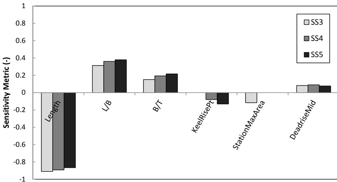
Figure 14. Sensitivity analysis results for the HSV's Total Resistance per tonne Displacement for each sea state
