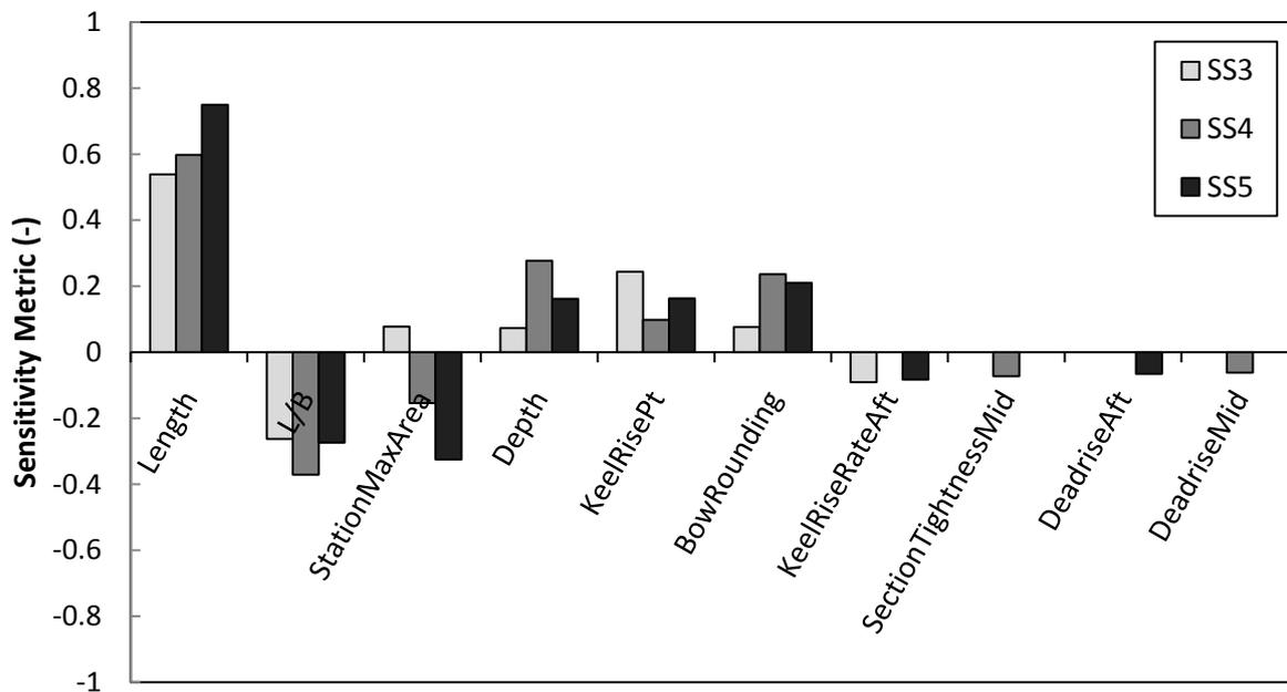
Figure 13. Sensitivity analysis results for the HSV's transit operability for each sea state
