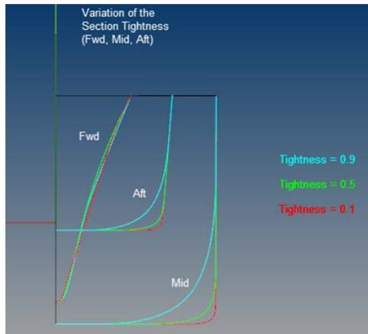
Figure A5. Body Plan view detailing use of the Section Tightness Aft, Mid and Fwd hull design variables
