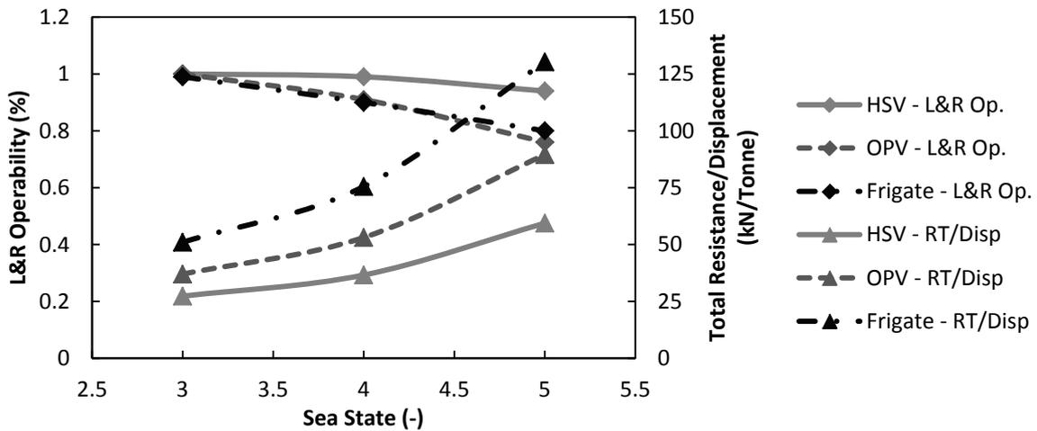
Figure 11. Optimal performances with respect to L&R operability and Total Resistance per tonne Displacement @ 14 knots for each vessel type for increasing sea state
