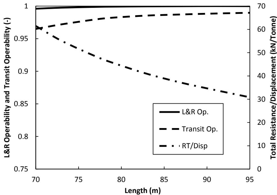
Figure 15. Response Surface Models of the HSV's length with respect to each of the three KPPs in sea state 3
