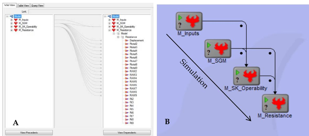
Figure 2 (A) Linkages between models allowing the transfer of data between inputs and outputs of separate models; (B) Simulation workflow – simplified view of integrated models
