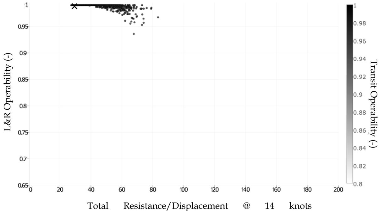
Figure 4. Scatter plot of the hydrographic survey vessel type hullform design space in SS3 illustrating the relationship between L&R operability and Total Resistance per tonne Displacement at 14 knots. Colour gradient represents the respective Transit operability.
