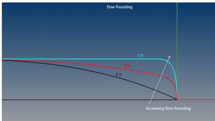
Figure A10. Plan view detailing the use of the Bow Rounding hull design variable
