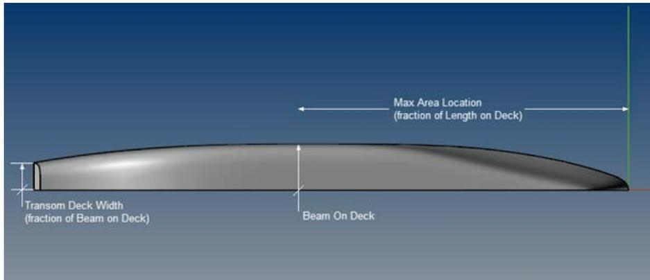
Figure A4. Plan view detailing the following hull design variables: Max Area Location, Beam (used for L/B) and Transom Deck Width.
