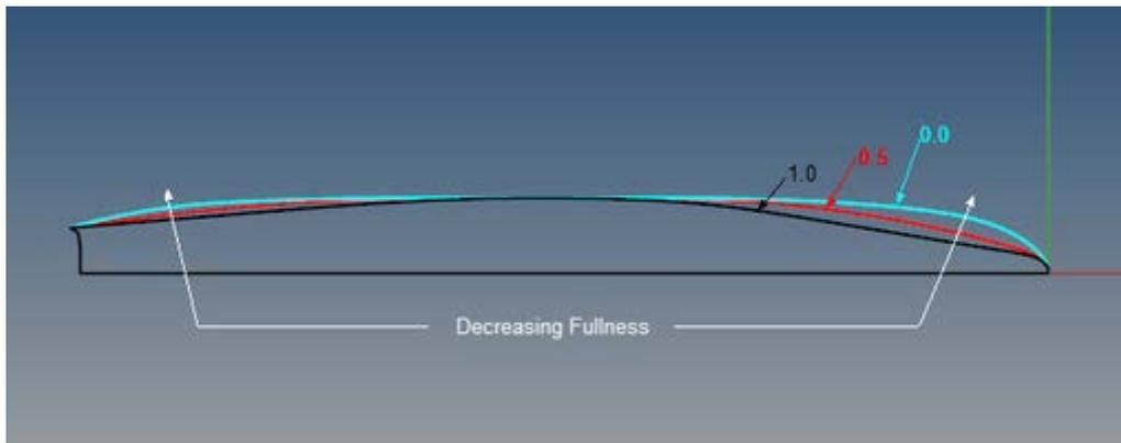
Figure A9. Plan view detailing the use of the Fullness hull design variable
