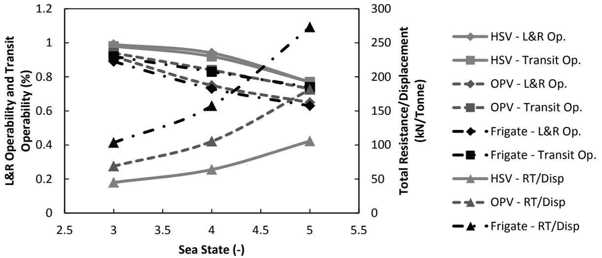
Figure 10. Mean performance of each KPP for each vessel type for increasing sea state
