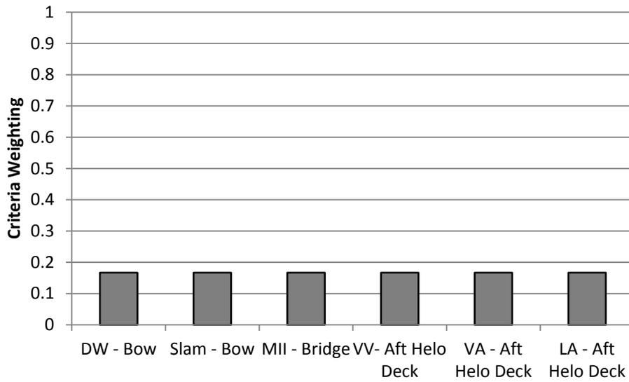
Figure B4. Weightings for each criterion at their respective locations for the transit seakeeping operability; Deck Wetness (DW), Vertical Velocity (VV), Vertical Acceleration (VA) and Lateral Acceleration (LA)
