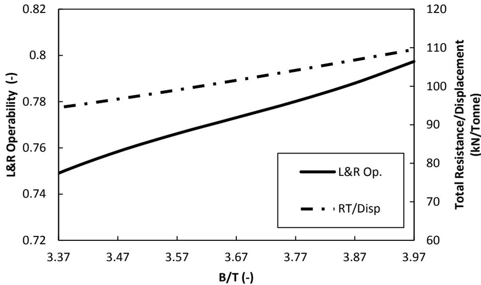
Figure 18. Response Surface Models of the HSV's B/T with respect to the L&R operability and Total Resistance per tonne Displacement in sea state 5
