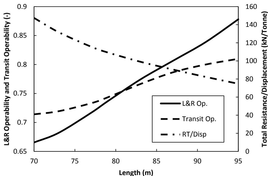
Figure 17. Response Surface Models of the HSV's length with respect to each of the three KPPs in sea state 5
