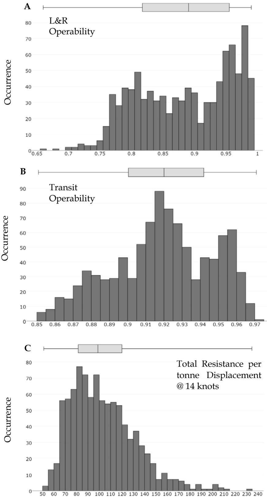
Figure 9. Histogram plots of the frigate vessel hullform in SS3 for: (A) L&R operability; (B) Transit Operability; (C) Total Resistance per tonne Displacement at 14 knots
