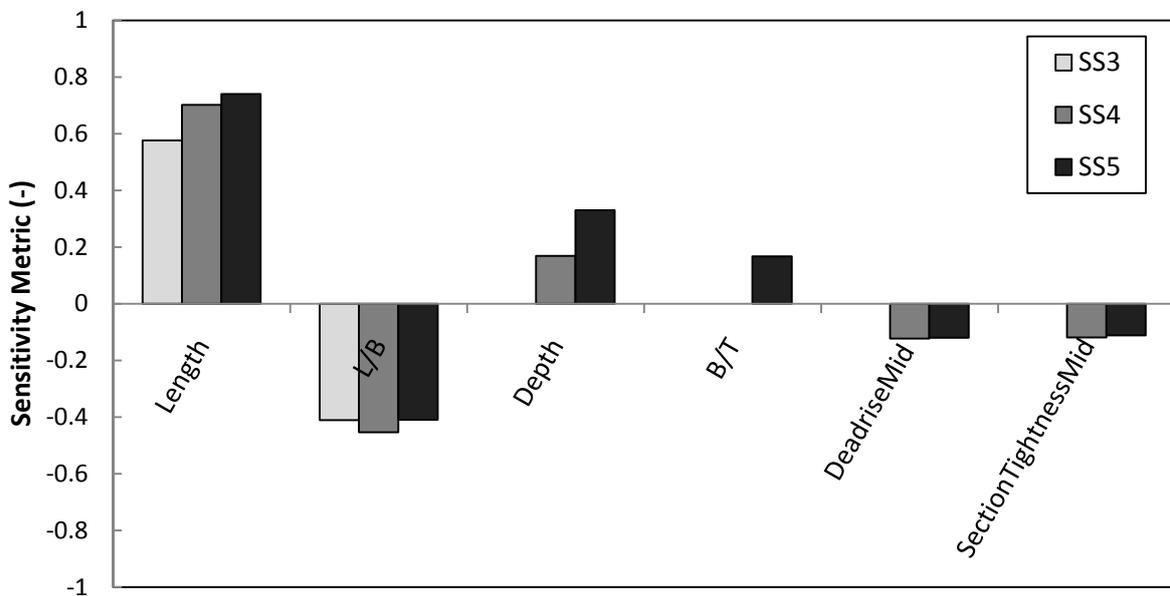
Figure 12. Sensitivity analysis results for the HSV's L&R operability for each sea state
