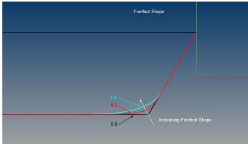
Figure A8. Profile view detailing the use of the Forefoot Shape hull design variable
