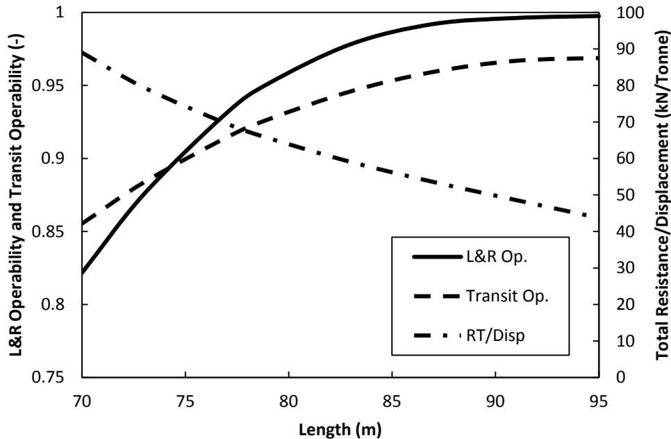
Figure 16. Response Surface Models of the HSV's length with respect to each of the three KPPs in sea state 4
