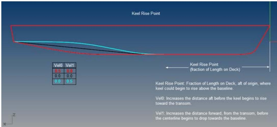
Figure A6. Profile view detailing use of the Keel Rise Point hull design variable
