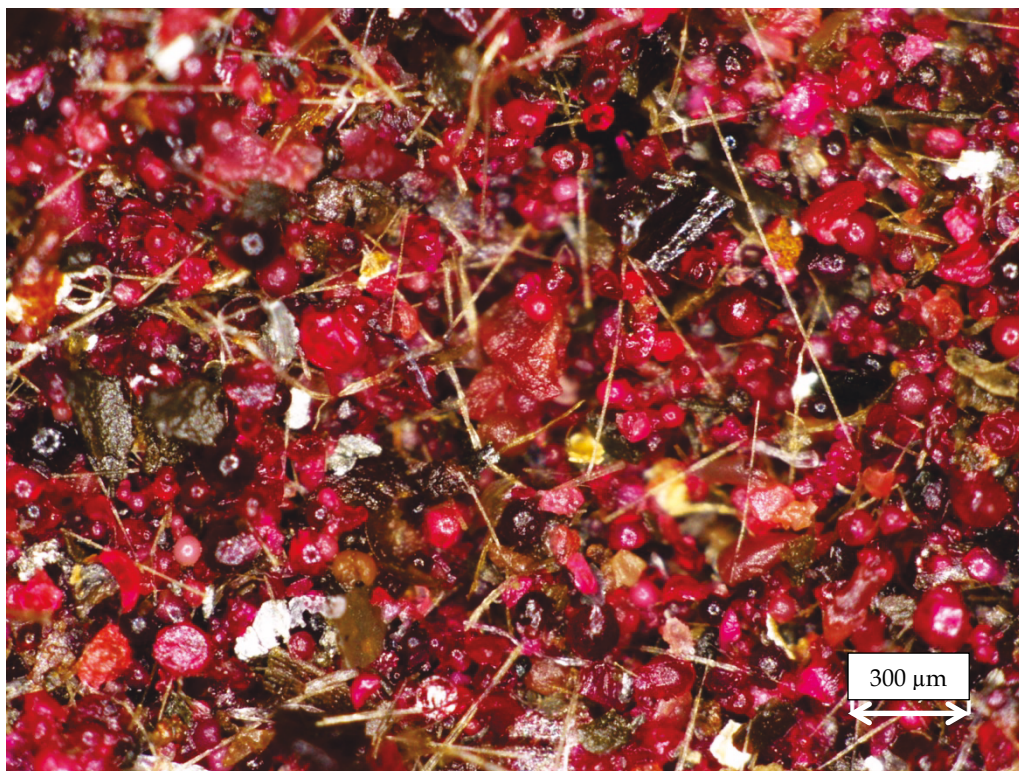
Figure 9: Filter debris extracted from A40-011 ESN 6534 showing extensive Al 2 O 3 coated in quinizarate
