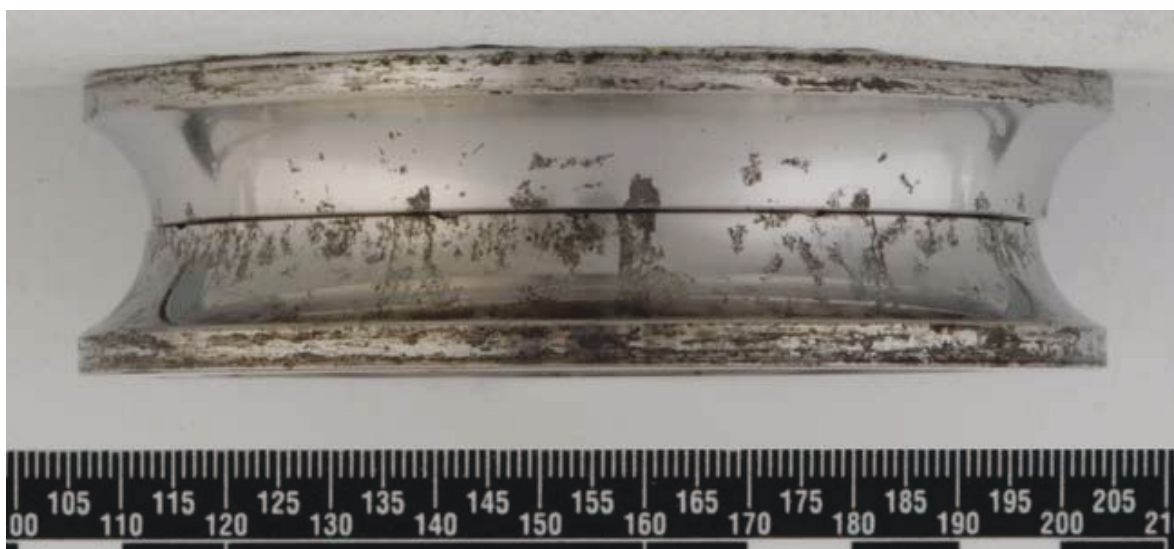
Figure 28: Split inner raceway showing extensive corrosion on the running surface and landings
