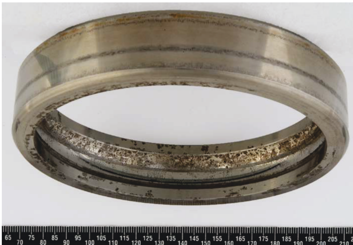
Figure 29: Outer raceway showing extensive corrosion on the running surface and various landings
