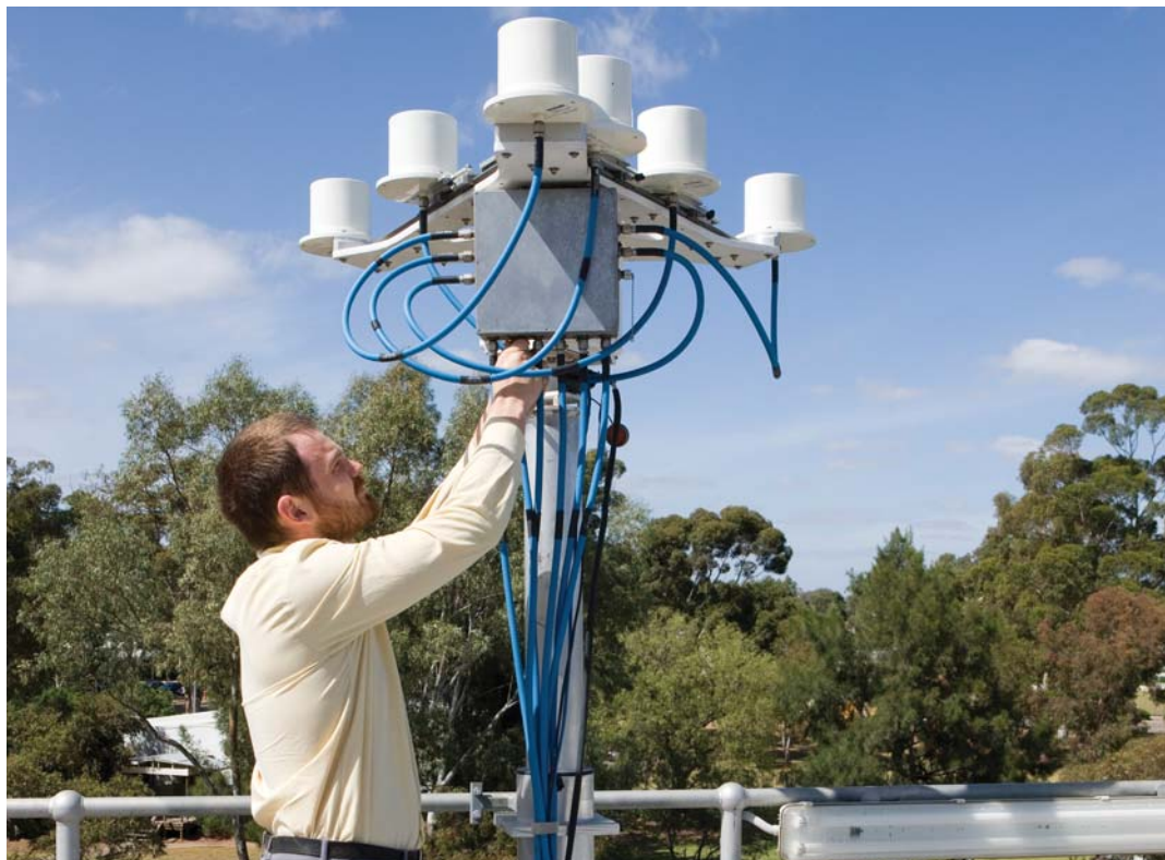
Pev Hall connecting RF cables to an experimental wideband multi-channel direction-finding array used with the advanced multi-channel receiver system.
