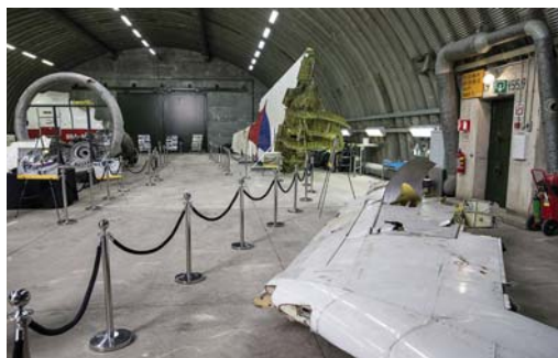
Mapping the wreckage for reconstruction to analyse how MH17 was destroyed.
