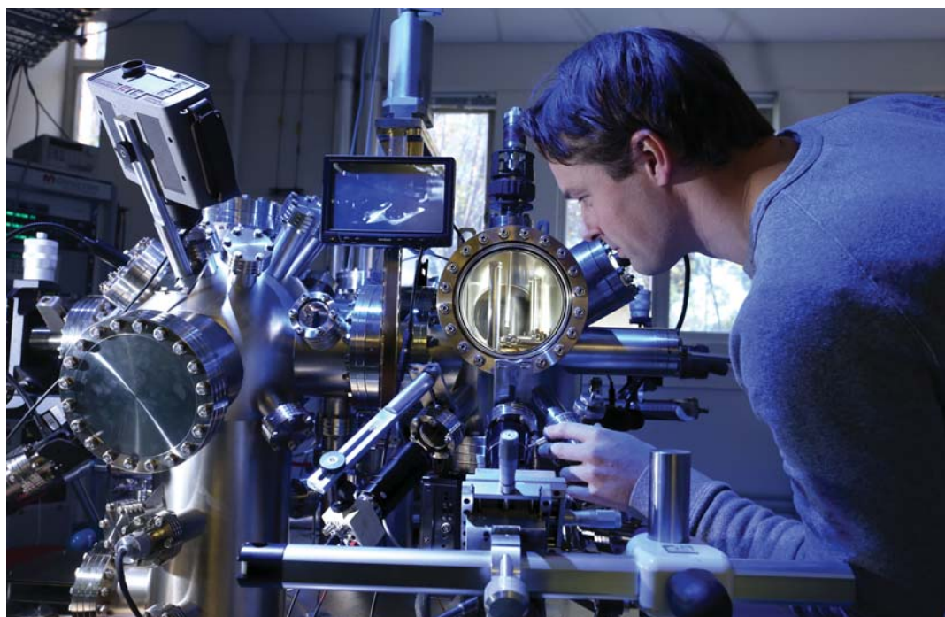
Operation of the scanning probe microscope used to position single phosphorus atom qubits in silicon.
