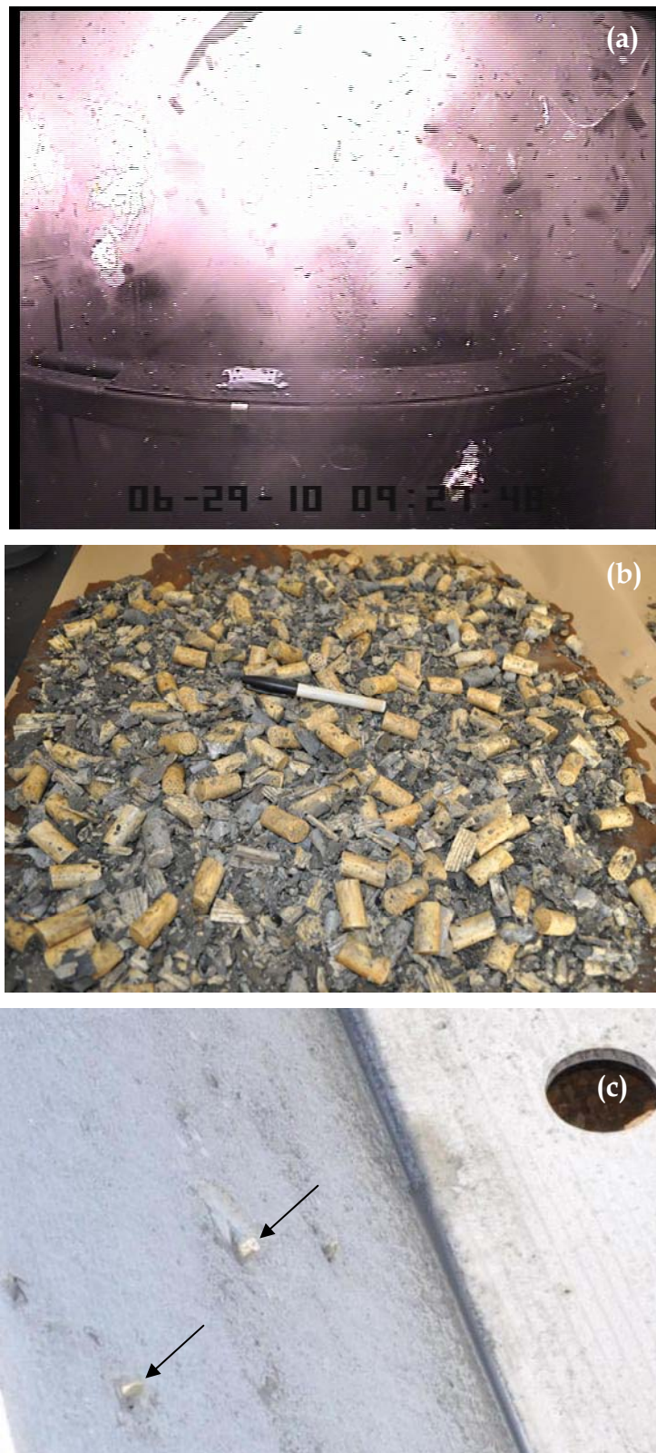
Figure 42: (a) Ejecta dispersion during Experiment 4, image from view A; (b) Post experiment propellant grain and grain fragments from Experiment 13; (c) Propellant shards lodged in flash bulb reflector, Experiment 13.
