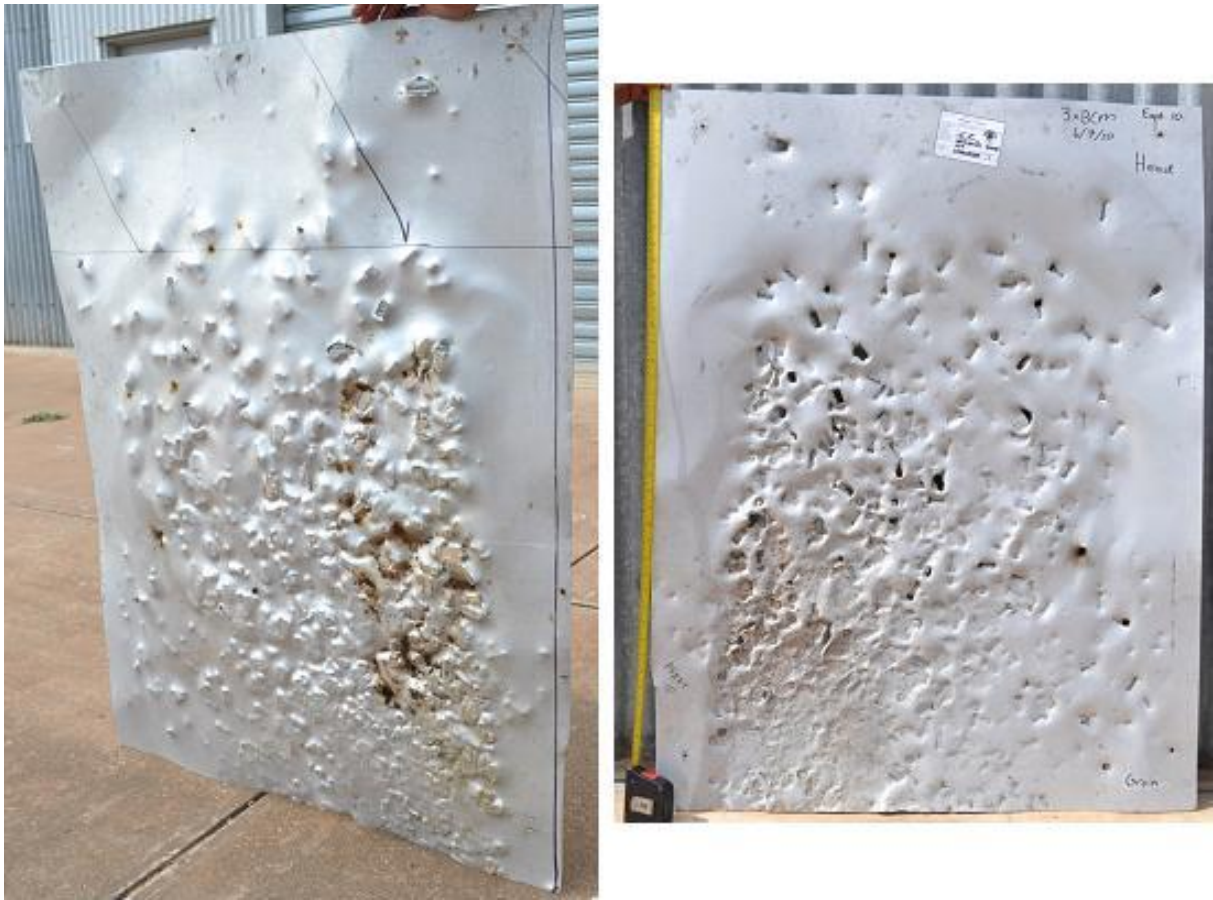
Figure 45: 1 mm thick 1.2 x 0.9 m Al witness plate used to assess ejecta dispersion for a 3xBCM configuration, Experiment 10. LHS image: witness plate viewed from behind. RHS image: view from front. Distance from top of propelling charge storage tube to witness plate was 1914 mm.
