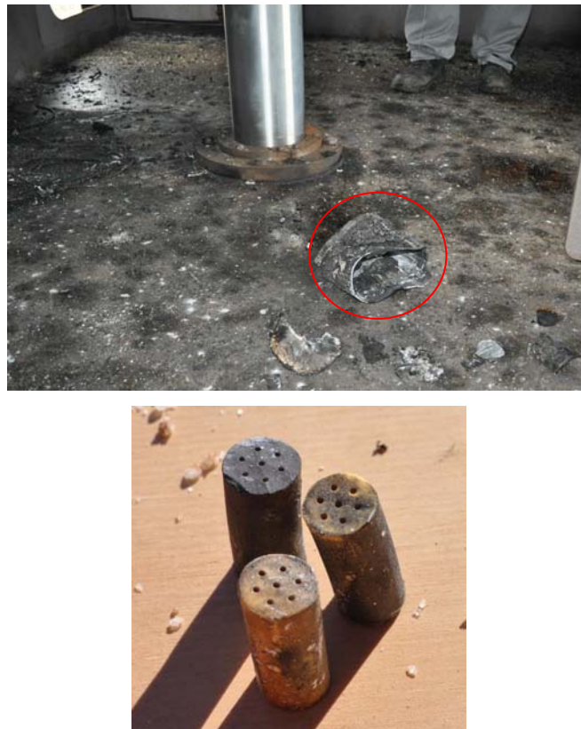
Figure 29: Burnt out combustible module case shell from Experiment 4 (top) and three propellant grains showing varying levels of outer graphite layer coating consumption collected from outside the trials structure in Experiment 1 (bottom).
