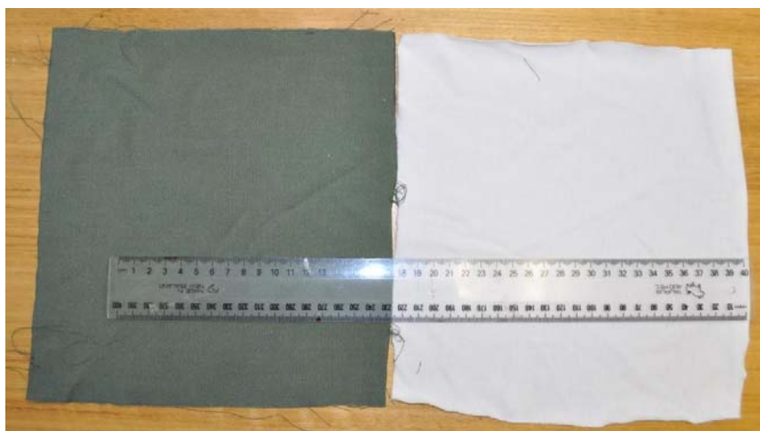
Figure 17: Nomex (left) and cotton (right) fabric swatches prepared for the trial
