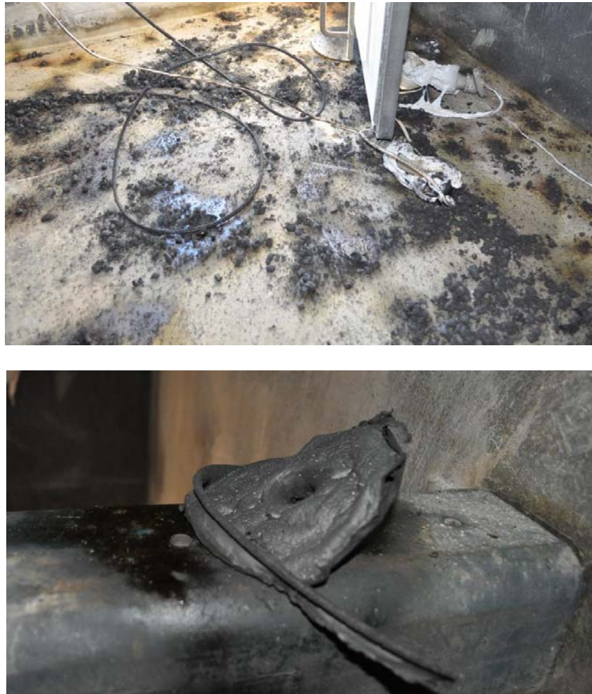
Figure 34: Carbonaceous propellant residue (top) and portion of burnt out combustible case (bottom) from Experiment 9
