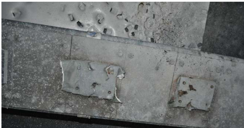
Figure 51: Ejecta damage to Person C in Experiment 13
