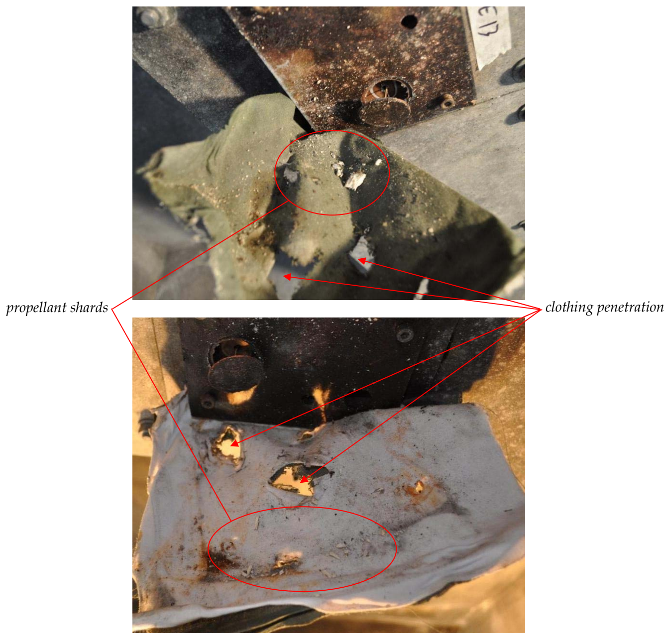
Figure 46: Propellant penetration through the clothing of Person C groin (top) and chest (bottom). Photo from Experiment 13.
