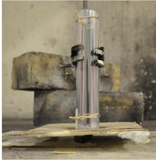
Figure 24: Experimental setup for configuration 2. The match-head can be seen below the cardboard sheet in-line with the plastic tube.
