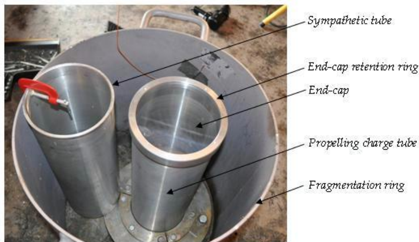
Figure 20: Propelling charge tube configuration for sympathetic fragmentation effect assessment
