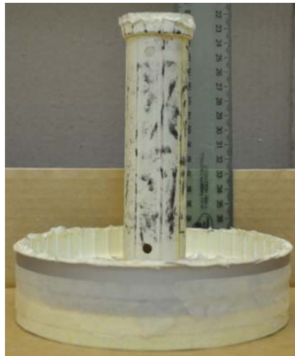
Figure 25: Image of the cut away combustible case used in configuration 3. The holes in the centre-core tube are also visible. The ruler markings are in cm.
