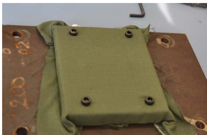
Figure 18: Instrumentation board covered with a cotton and Nomex fabric swatch
