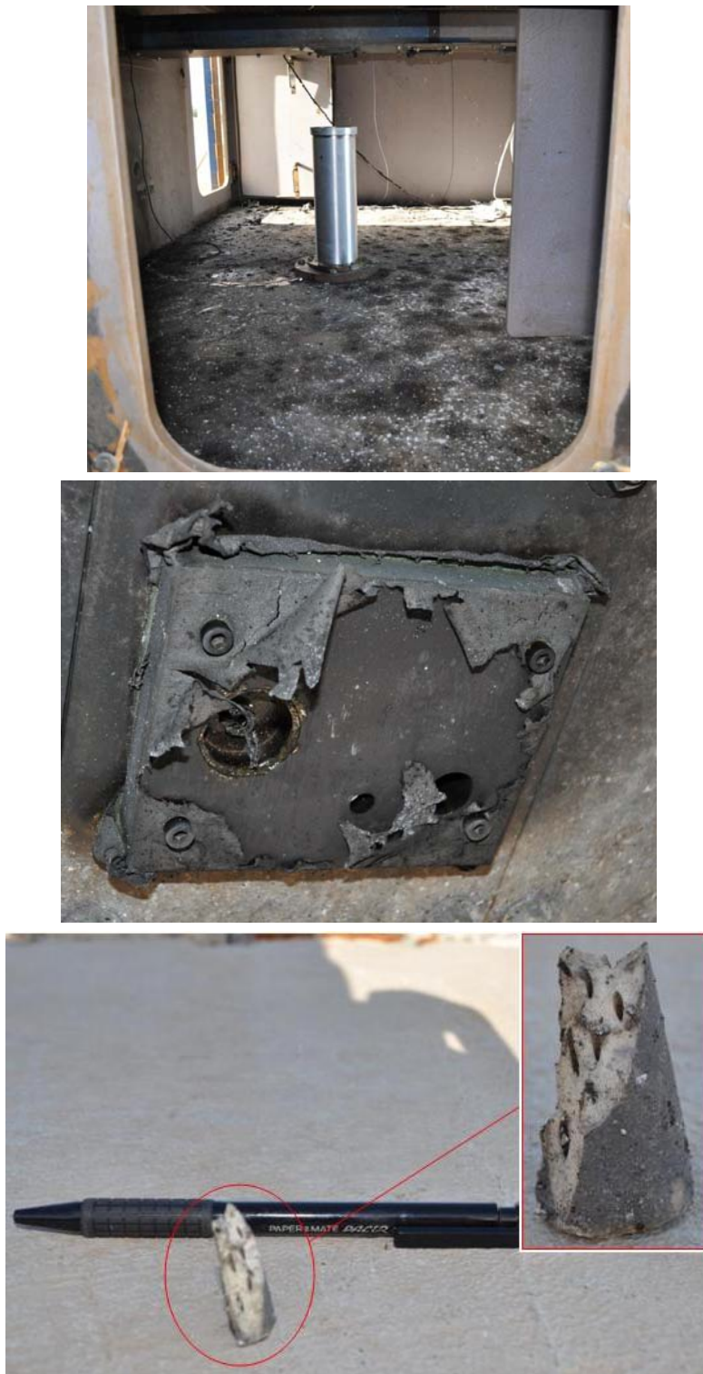
Figure 32: (top) Burn marks on floor of trial structure highlight the widespread burning of propellant throughout the structure; (middle) Person C groin showing the loss of the copper disc sensor and the destruction of the Nomex clothing initially protecting the groin; (bottom) Fractured propellant grain collected from outside the trials structure near the vent hatch.
