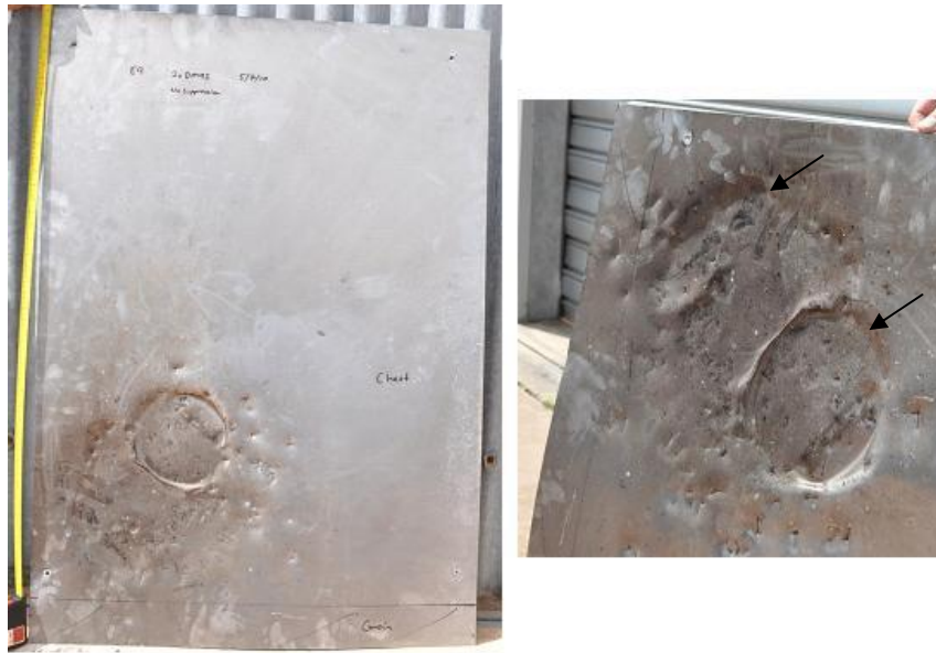
Figure 53: 1 mm thick Al witness plate used to assess ejecta dispersion for a 2xATC configuration, Experiment 9. RHS image shows close up view of the two circular impressions left by the module and end-cap. Distance from top of propelling charge storage tube to witness plate was 1914 mm.
