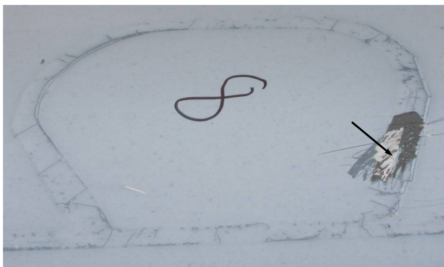
Figure C.2: Photograph of a patch with sufficient sealant removed to identify the blue FM300 adhesive (arrowed)
