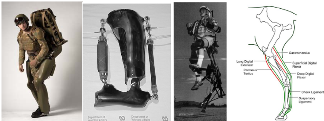
Figure 12: [a] Powered Exoskeleton, [b] Powered Exotendon, [c] Unpowered Exoskeleton & [d] Horse Tendon
