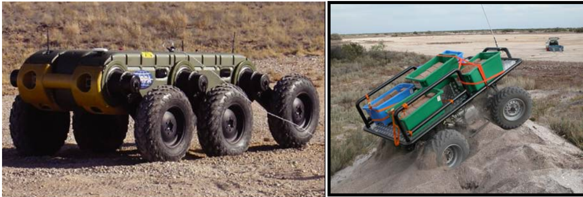
Figure 16: The MULE 8 (left) & the DSTO MAULER (right) carrying 250 kg over sand.
