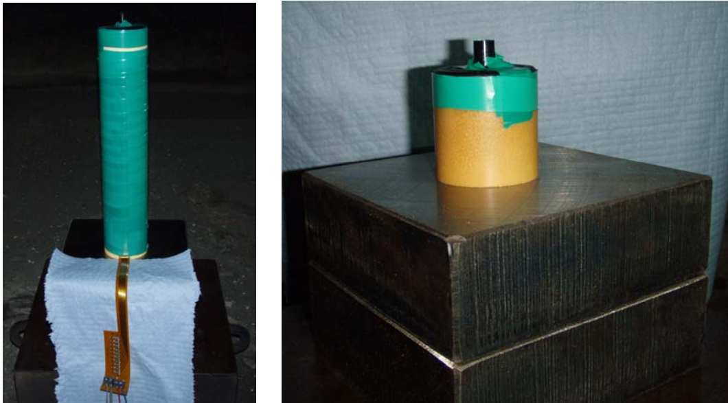
Figure 1: (a) VoD charge configuration (b) Single donor dent test setup in the DSTO HEFC
