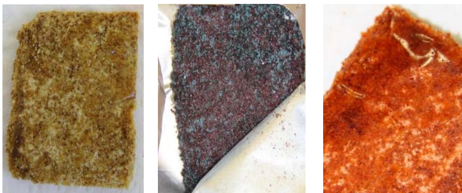
Figure 15. Sports Drink Powder, NEB & caking after 28 days storage at 50 °C for (left to right) Lemon/Lime, Grape and Orange flavours.
