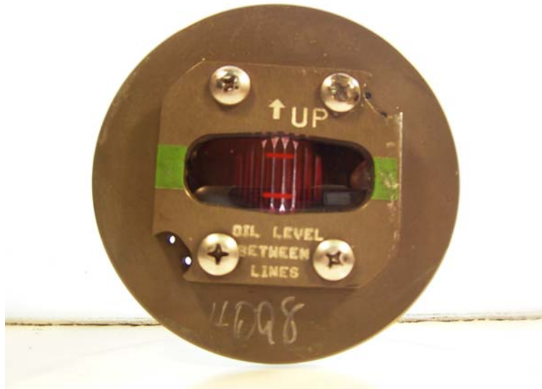
Figure B1. Sight glass from a Black Hawk, rear lit showing obscuration with red stain
