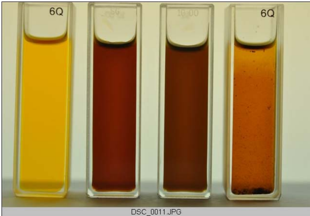
Figure A5. Oil samples from left to right: Fresh Mobil Jet Oil II; A25-107 TRGB; A25-204 TRGB; A25-107 TRGB with precipitate (samples from 2005 archive photo)
