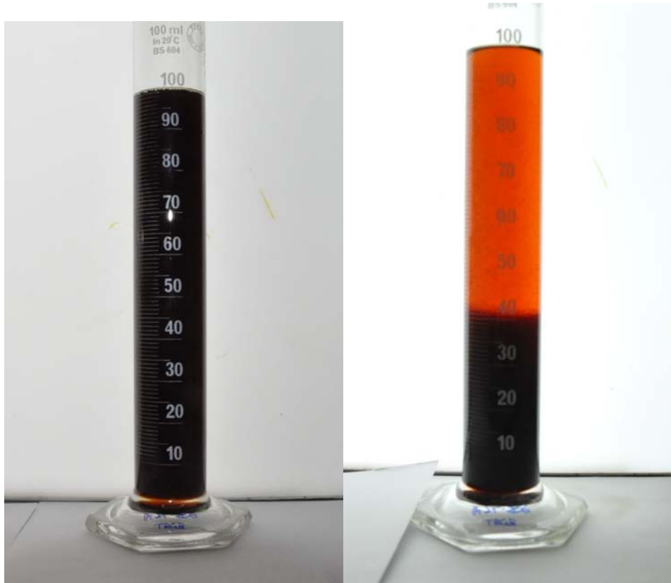
Figures A1 and A2. A25-206 TRGB oil before and after 48 hours standing
