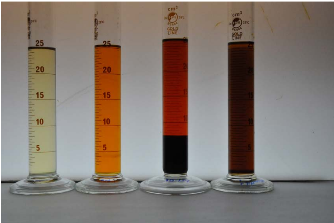
Figure A4. MIL-PRF-23699 Fluids after 48 hours standing.
