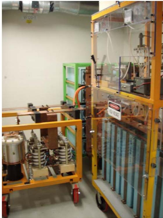
Figure 2. The picture shows some of the components of the PPS. In the foreground are 5 vertically stacked capacitors above which sits safety and control features. The left rear shows the diode clamp and the cylindrical spark gap switch.
