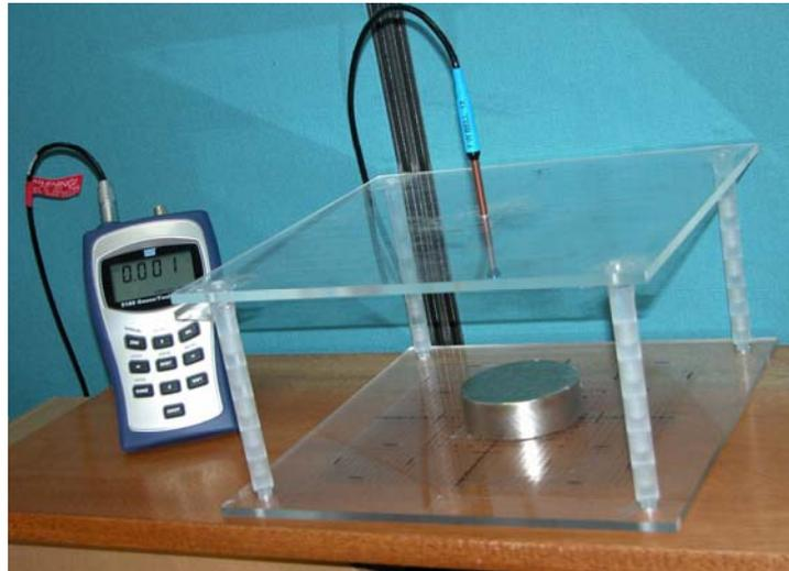
*Figure 1. Rare earth disc magnet undergoing field measurement*
