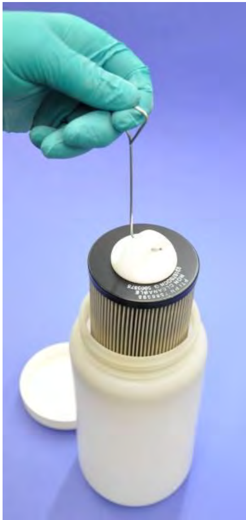
Figure 5: Plugged filter element being lowered into the cylindrical extraction container.
