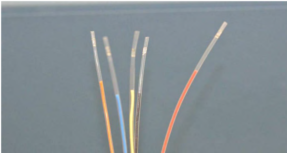
Figure 37: Test straws showing embedded particles of known size
