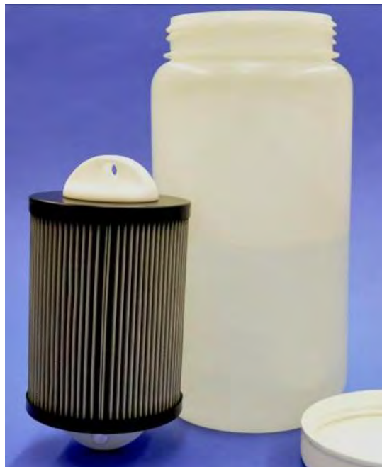
Figure 4: Plugged F117 oil filter and extraction container
