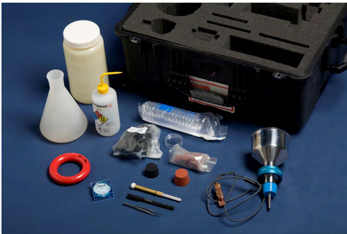
Figure 2: Contents of Filter Debris Extraction Kit
