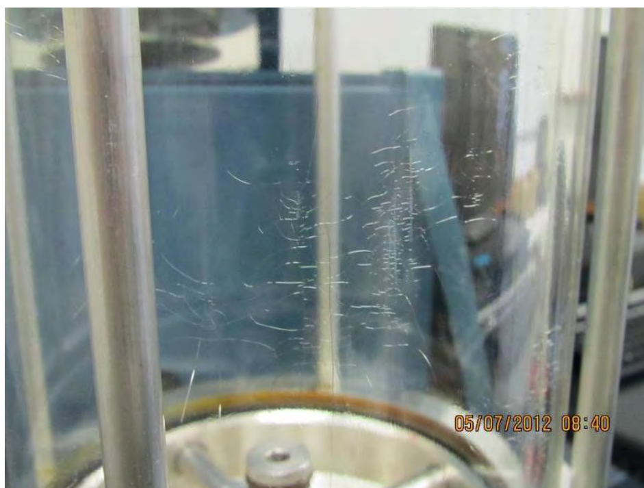
Figure 34: Wash Housing showing crazing
