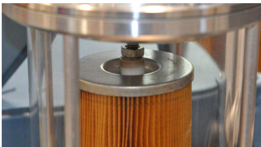
Figure 28: Top of T56 ESF in the FC290 showing the Wash Housing plunger bearing directly onto the solid top of the filter element.
