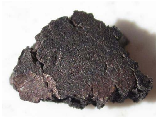
Figure 7 The optical probe-facing side of a fragment of the metal disk recovered after the explosive event. The fragment's width is about 1 cm.
