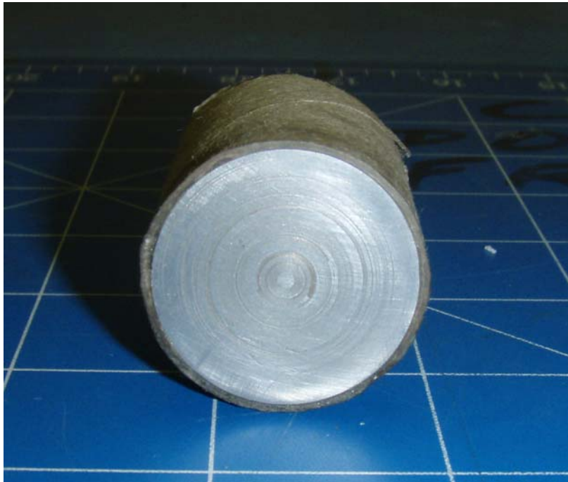
Figure 1 View of a typical explosive charge assembly from the steel disk end. The diameter of the steel disk is 30 mm and the length of the assembly is 35 mm (30 mm charge and 5 mm steel disk) encased in a cardboard tube.
