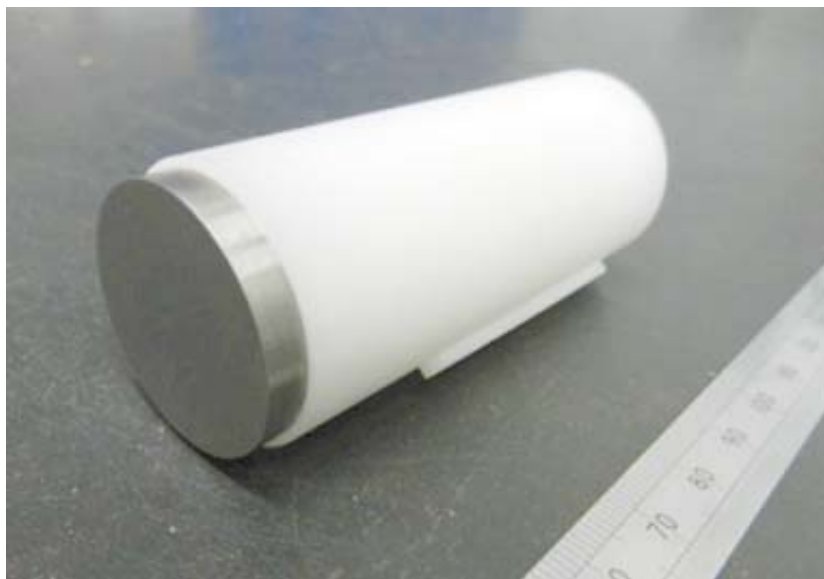
Figure 1 Sabot, 29.7 mm diameter and 70 mm length, made from acetyl homopolymer with an aluminium flyer plate
