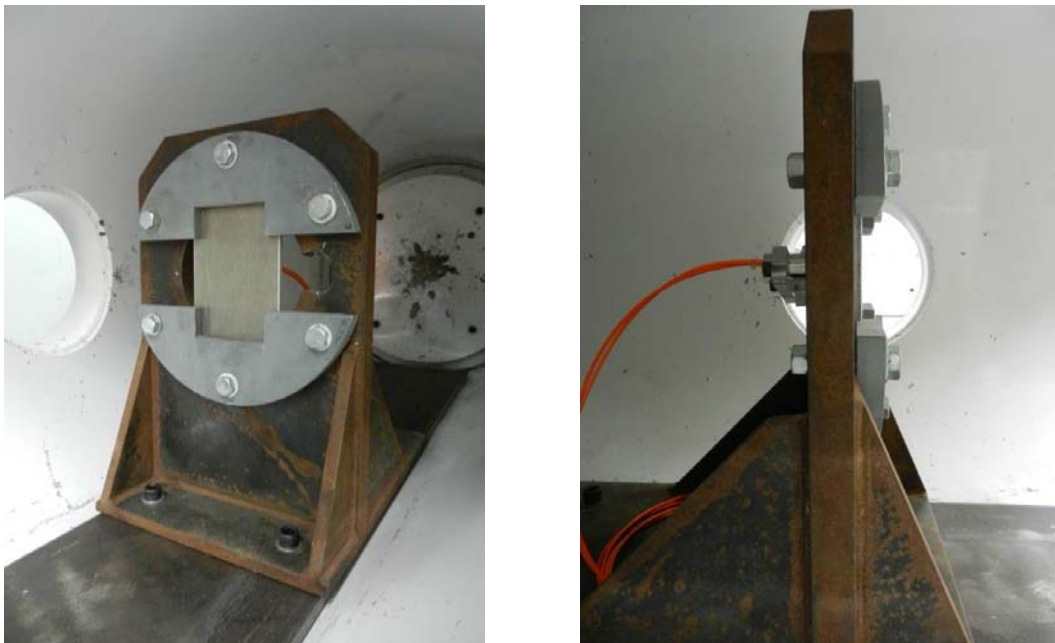
Figure 4 Front and side views of the experimental set-up (target mount)
