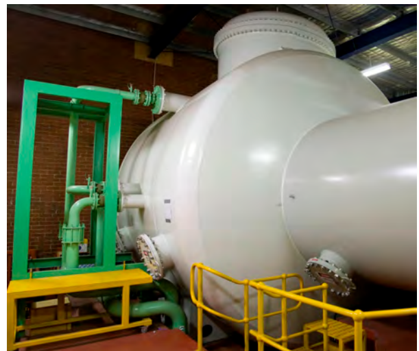
Figure 10: Settling chamber casing and heat exchanger pipework
