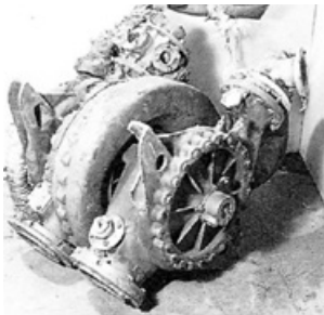
The steam-driven turbine and centrifugal propellant pumps from a recovered V2, December 1944. (RAE)
