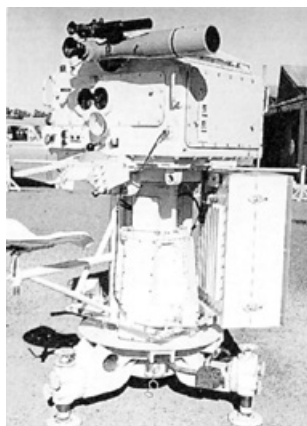
An optical tracker, usually known as an X-tracker.
