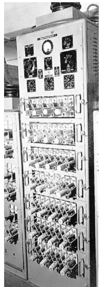
The No. 2 analog impact predictor, which used thermionic vacuum tubes
