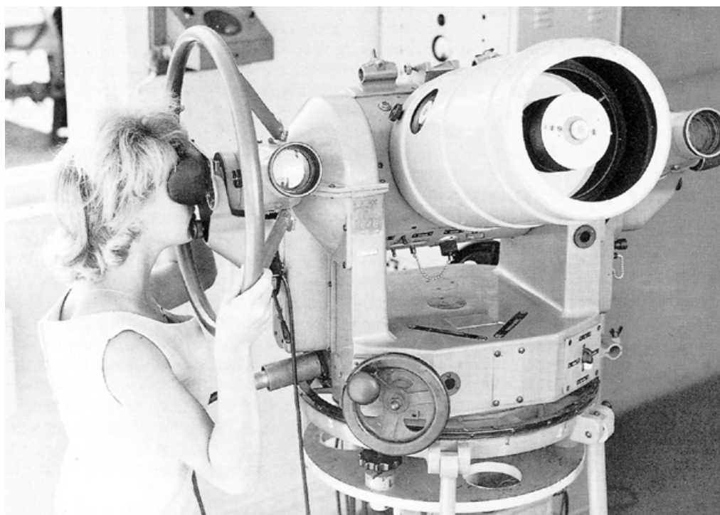
A KTh52 Askania fitted with direct acting handwheel and 1000 millimetre mirror lens.
