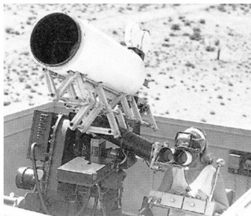
Far left: 'IOTER', an early WRE servo-controlled powered mount for long distance photography.
