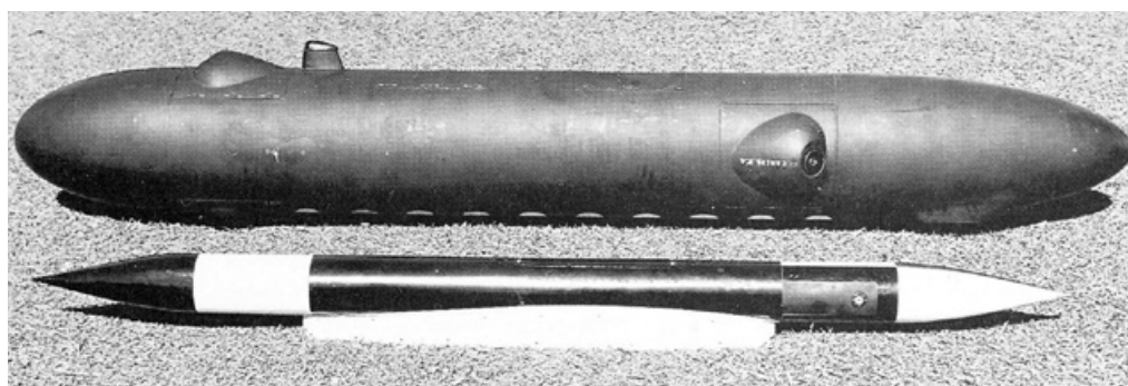
A 14-centimetre diameter pod alongside the old 38-centimetre pod designed for GW2 cameras.
