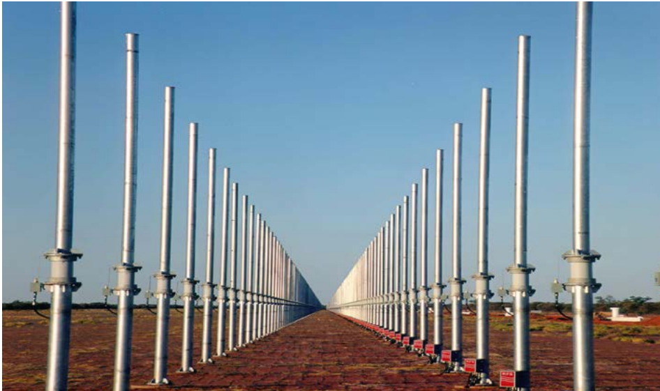
The receive array uses fat monopoles to improve performance across the high frequency band and to reduce the effect of wind induced motion on the received signals.
