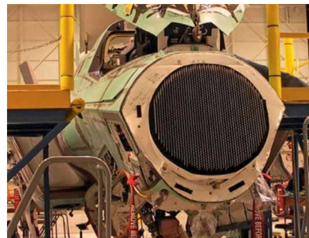
The APG-81 AESA radar represents the primary long-range sensor system on the F-35 and at the time represented a significant advancement on any other combat aircraft radar, including that on the earlier USAF F-22.
