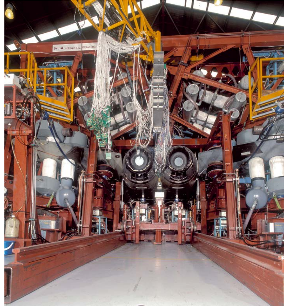
Looking at the back end of the FT46 test article in the completed IFOSTP rig at DSTO Fishermans Bend. The test article was slid into position via the rail system along the floor.
