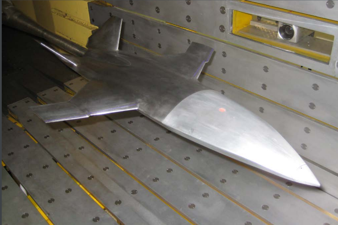
| Scale model of the Boeing ATS located in the transonic wind tunnel at DSTG Fishermans Bend in 2017.
