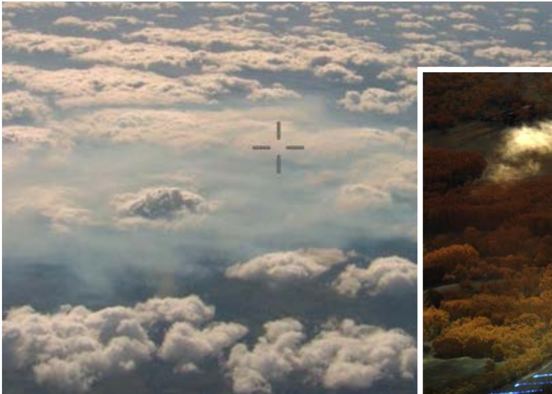
Smoke obscures the visible image (left) but the HSI shows the flames of a planned burn-off through the smoke (below).
