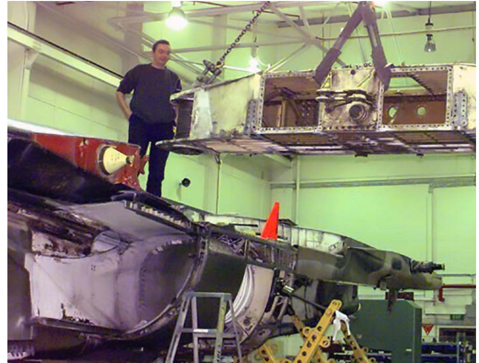
Removal of the wing carry through structure. The teardown concluded that this aircraft was representative of a 30+ year old aircraft in the RAAF fleet, and that it was in relatively good condition considering its age.
