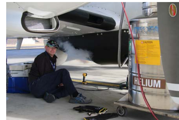
DSTG scientists calibrating hyperspectral sensors mounted under the DEAP Beechcraft 1900C at RAAF Edinburgh for a comparative trial in 2019 with a RAAF P-8A Poseidon. (Left to right): Dr Tim Bubner (DSTG Hyperspectral Lead), Steve Lang (DEAP Lead pilot), Merrilyn Fiebig (Project Lead) and Gavin Fowler (LWIR Sensor Technical Lead). In the right photo Gavin is cooling the LWIR sensors with Helium before take-off.
