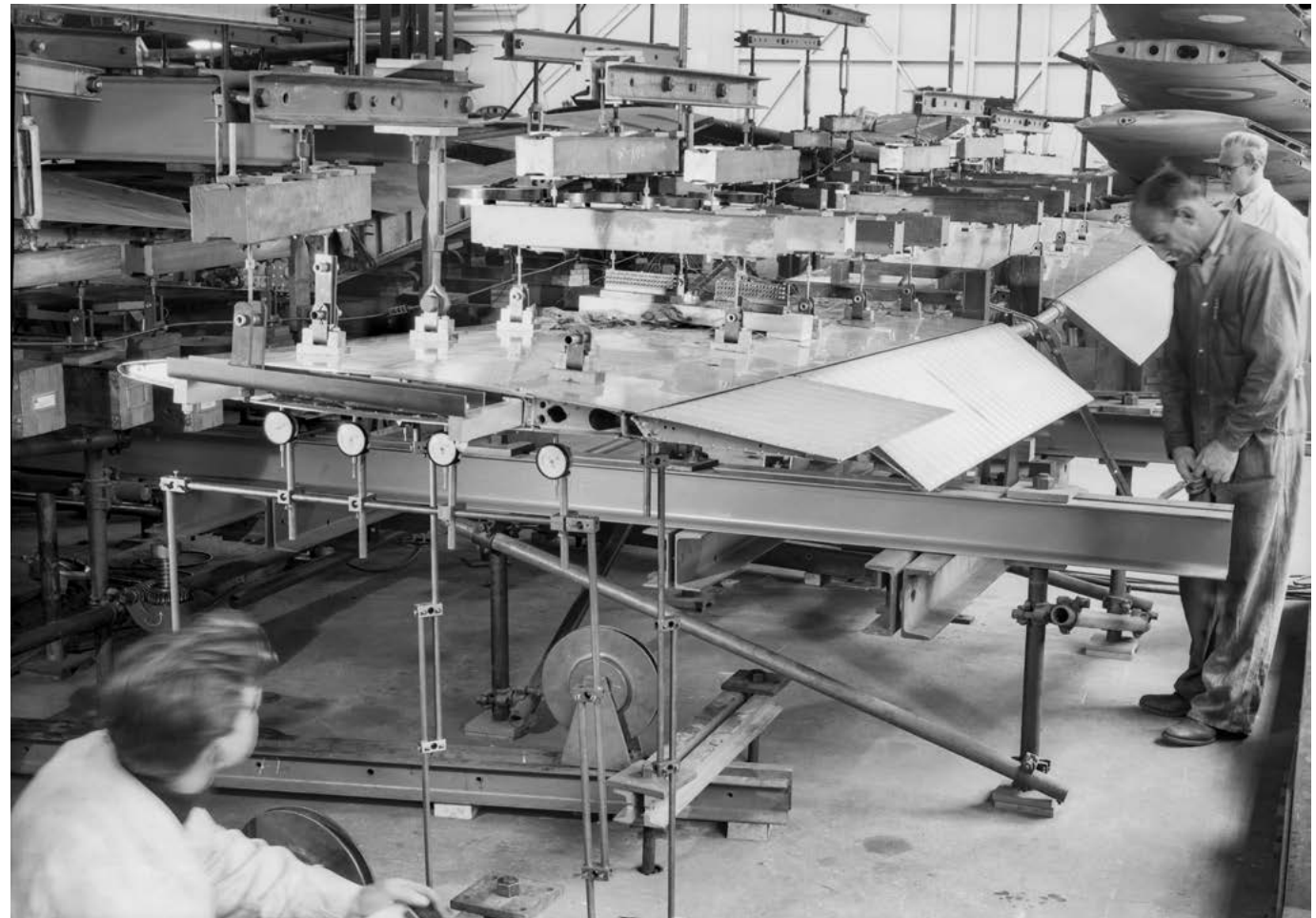
Static strength testing of a Jindivik wing at ARL, Fishermans Bend, October 1953. Note the stack of Mustang wings in the top right of the image.
