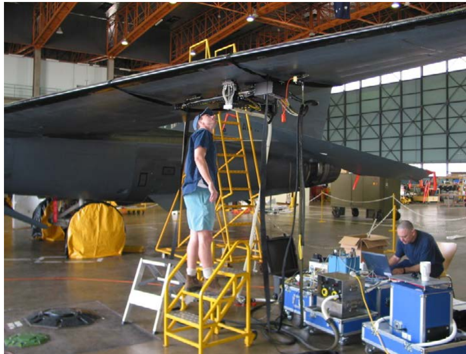
The F-WELD test article under high positive g loading at Fishermans Bend. This wing had been removed from USAF aircraft 72-1449 which took part in the Operation El Dorado Canyon air strikes against Libya in 1986.
