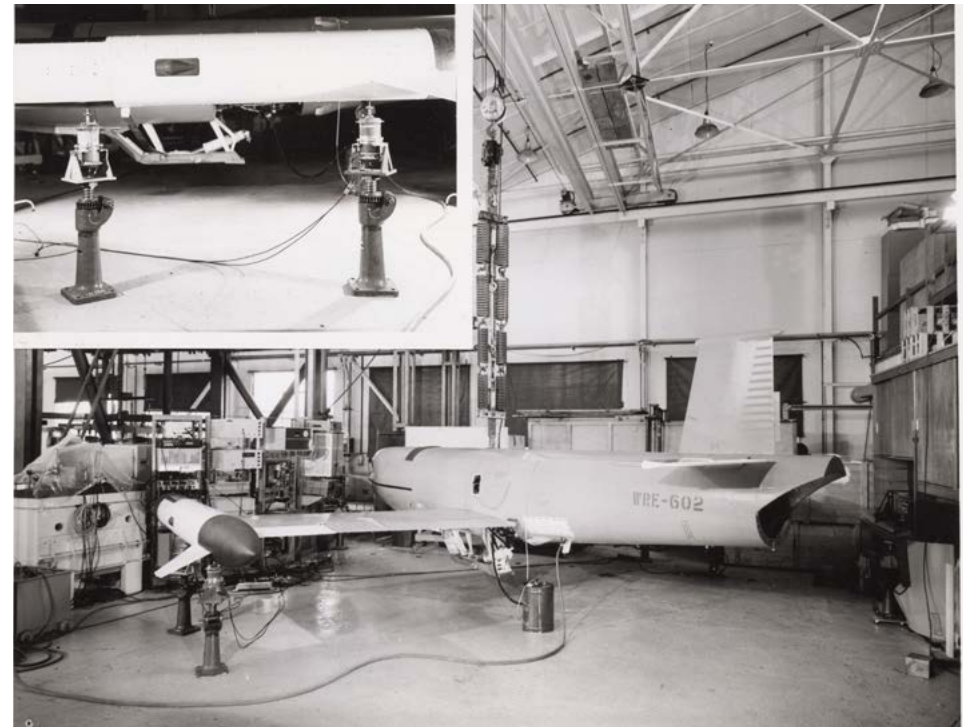
Jindivik Mk 3B WRE-602 undergoing ground vibration testing at Fishermans Bend, around 1970. Measurements of low frequency wing bending and torsion modes were made as the basis for the mathematical model of the aircraft's aeroelastic characteristics when fitted with Mk 7/8 wingtip pods. The inset (top left) shows the vibration module set up on the wingtip pods.
