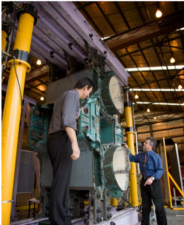
(Above) The HOWSAT test program at Fishermans Bend was successfully used to develop a through-life management strategy for the outer wing in RAAF service after interpretation of previous full-scale fatigue tests conducted overseas had proven futile.
