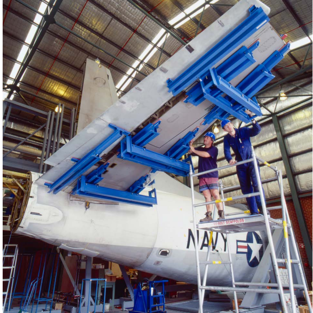
| P-3C empennage test set up.
