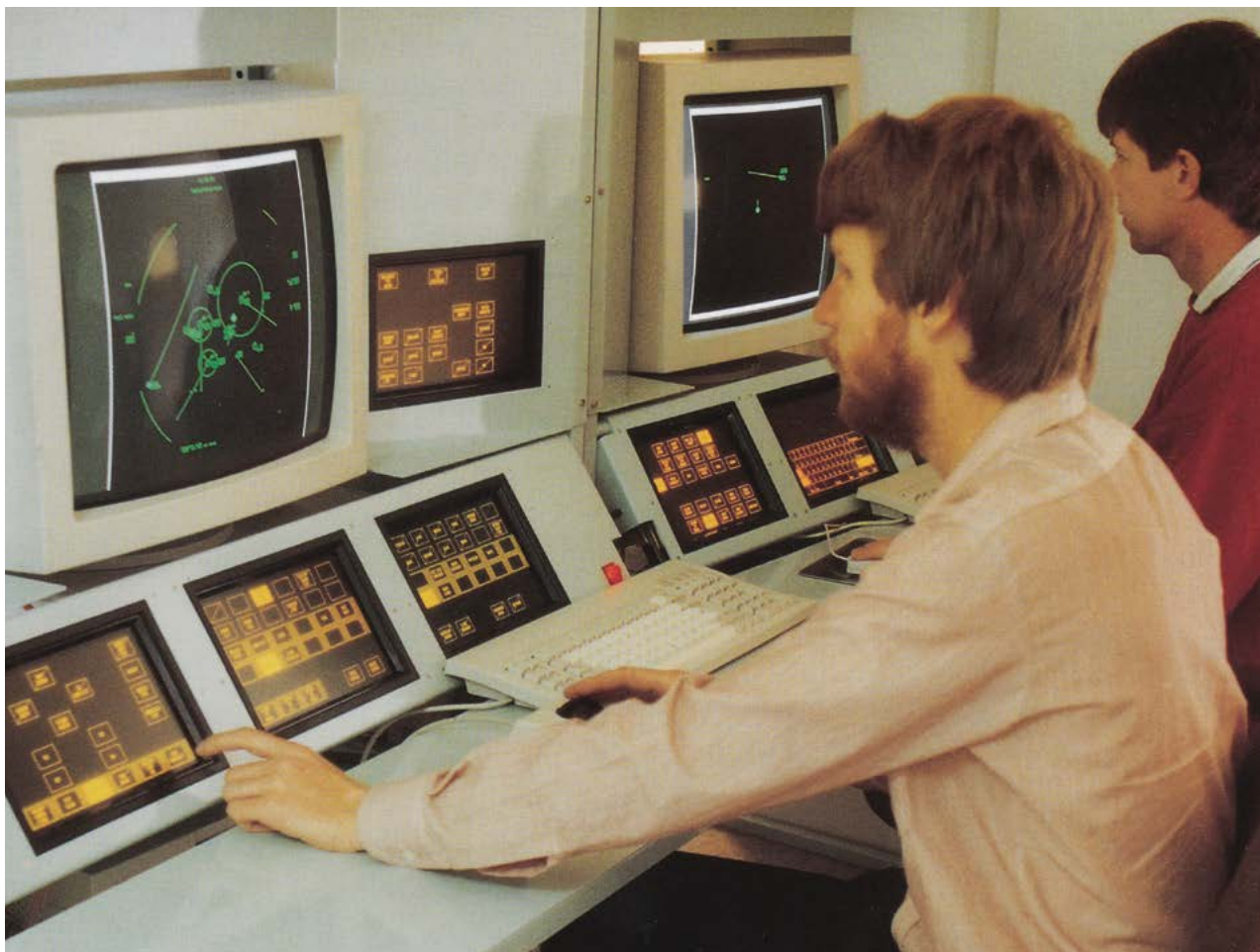
In 1991 the ORACL was a state-of-the-art research facility with Sun workstations running X Windows, track balls and keypads, and some of the first touch screen controllers representing future consoles for maritime patrol operators. Shown are DSTO engineers Peter Temple (nearer) and Mark Davies.
