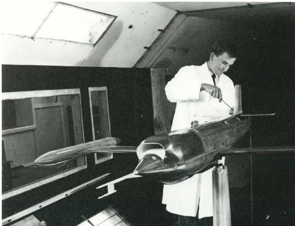
A quarter scale Jindivik model with Mk 7 wingtip fuel pods being prepared for testing in the low speed wind tunnel at Fishermans Bend, 1965.
