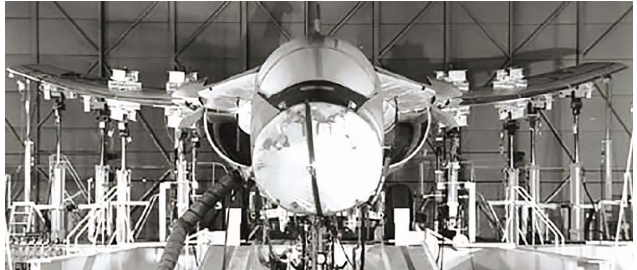
| F-111 CPLT – wings shown subjected to 7.33 g force up-loading whilst at a temperature of -40^{\circ} .
