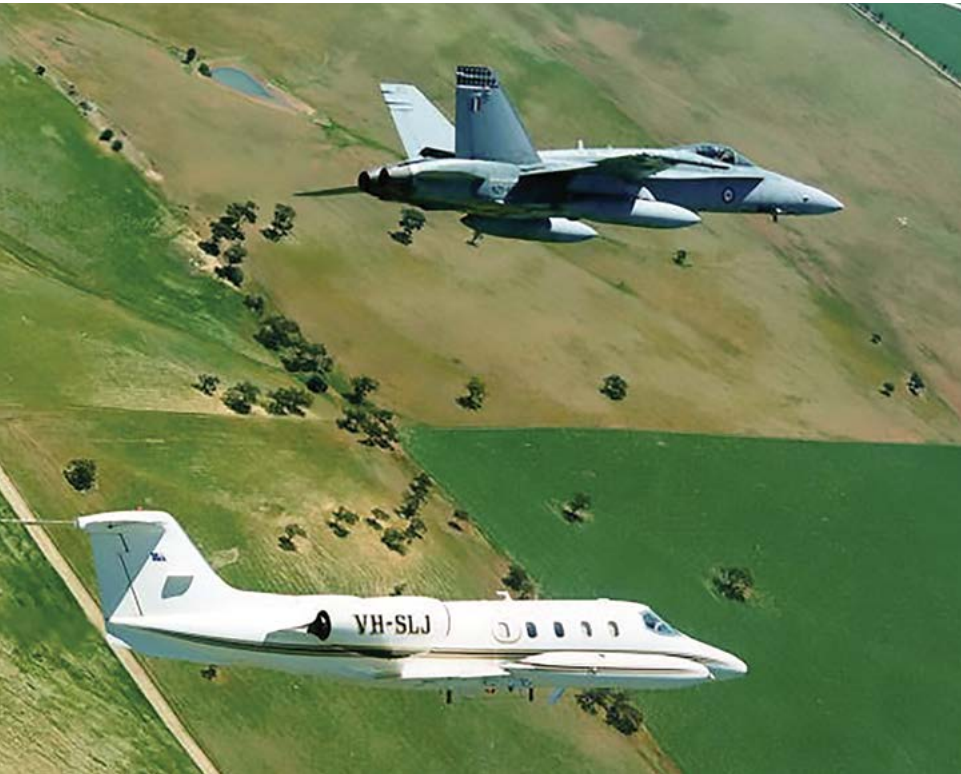
The Pel-Air Learjet VH-SLJ was modified to carry the ECM testbed for flight testing with an F/A-18A at RAAF Edinburgh.
