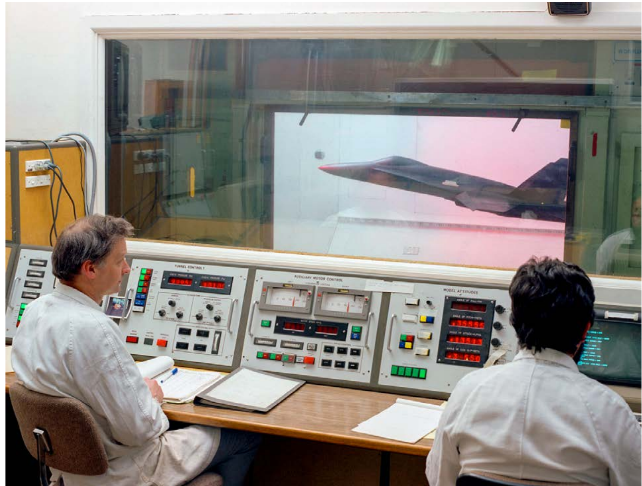
Dennis Carnell (left) and Alberto Gonzalez (right) at the controls of the low speed wind tunnel at Fishermans Bend, with the 1/9th scale Classic Hornet model undergoing aerodynamic measurement testing, circa 1990.
