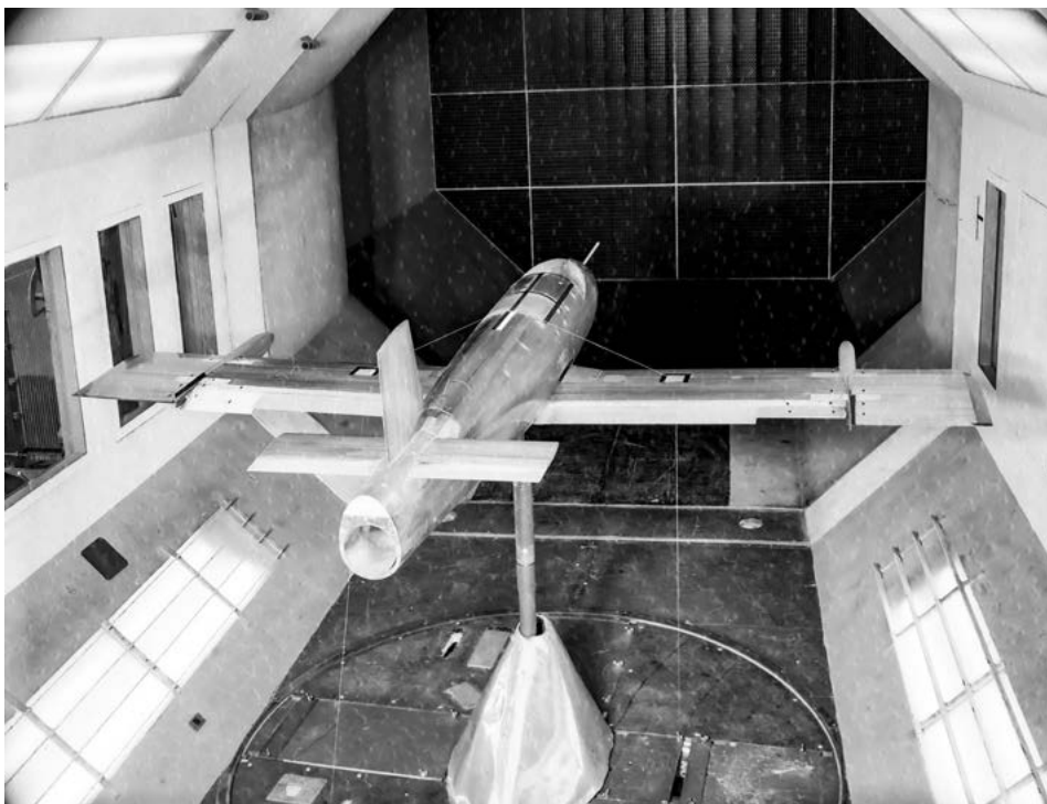
2/7th scale Jindivik wind tunnel model with Mk 3 pods and wing tip extensions undergoes testing in the 9' x 7' low speed wind tunnel, 1957.
