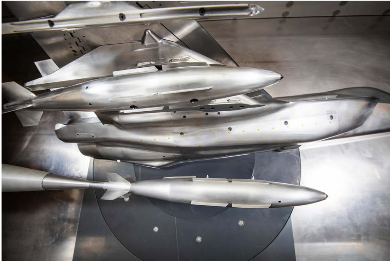
A model of a GBU-61 2000lb Joint Direct Attack Munition (JDAM) positioned below a partial F-35 model in the DSTG Transonic Wind Tunnel at Fishermans Bend in 2021.
