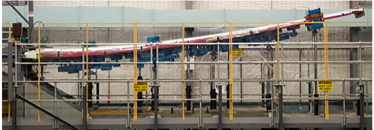
The F-WELD test article under high positive g loading at Fishermans Bend. This wing had been removed from USAF aircraft 72-1449 which took part in the Operation El Dorado Canyon air strikes against Libya in 1986.
