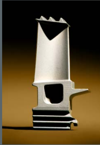
A new turbine blade from a late model T56 engine before undergoing test and inspection by DSTO.
