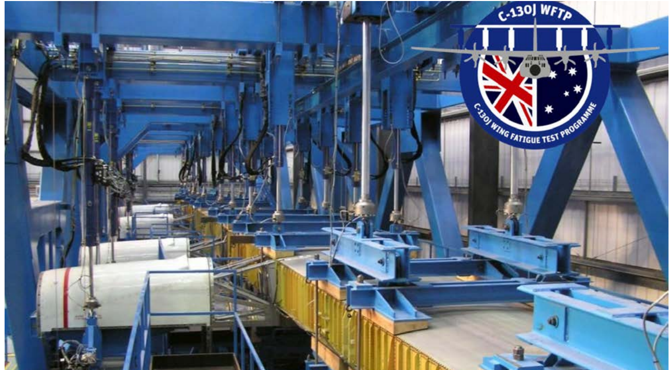
The C-130J-30 test article wing was a production wing sourced from Lockheed Martin Aero. Shown in the test rig at Marshall Aerospace, a total of 40 servo-hydraulic actuators applied the loads (24 on the wing, 3 per engine and 4 on the fuselage side walls) whilst an airbag was used under the centre wing carry through structure. This durability and damage tolerance test was completed according to the requirements of the US military specification JSSG-2006.
