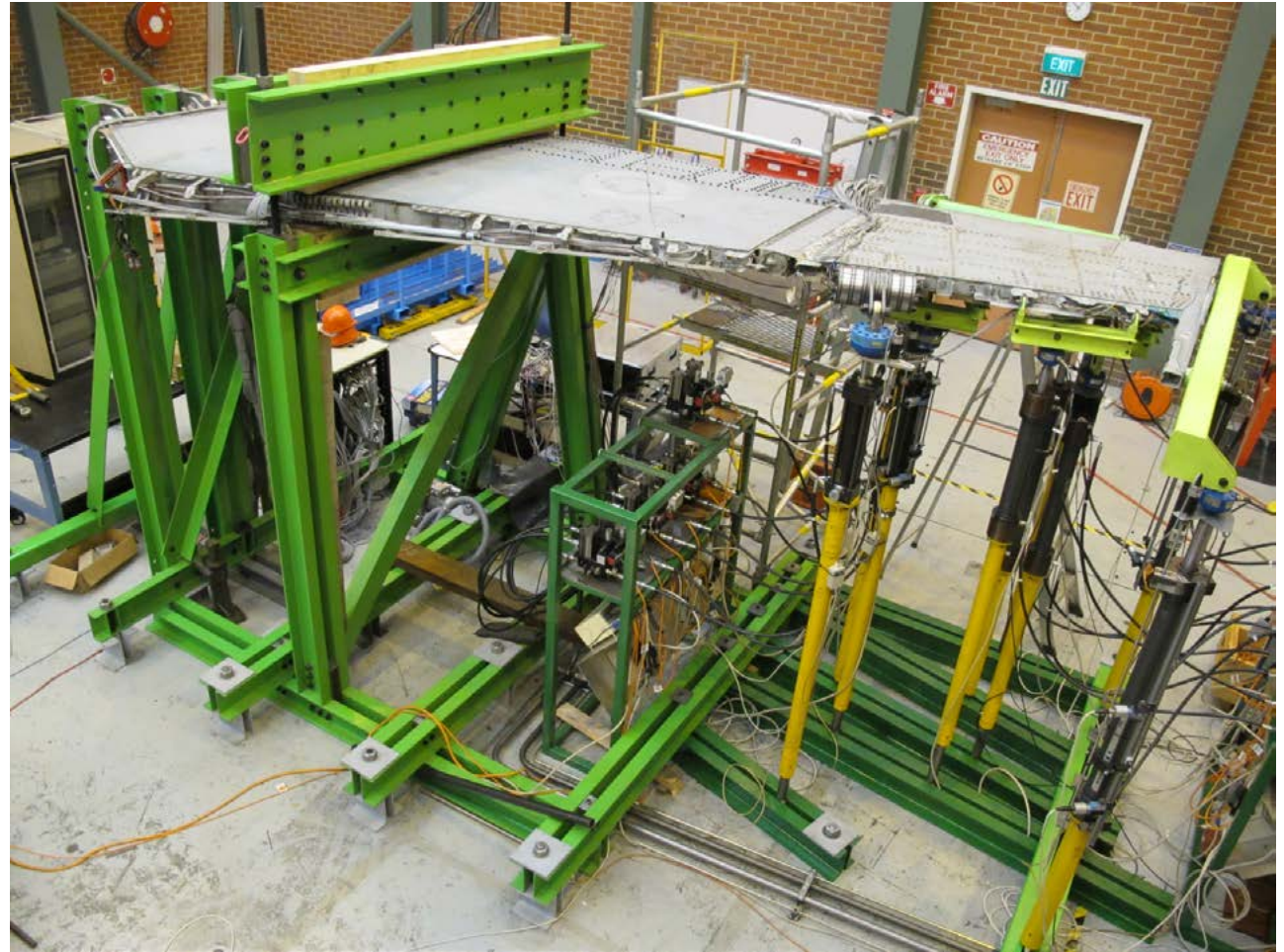
(Above) The HOWSAT test program at Fishermans Bend was successfully used to develop a through-life management strategy for the outer wing in RAAF service after interpretation of previous full-scale fatigue tests conducted overseas had proven futile.
